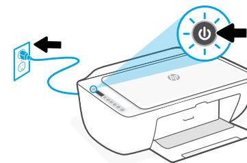
**EN** Plug in and turn on the printer.
