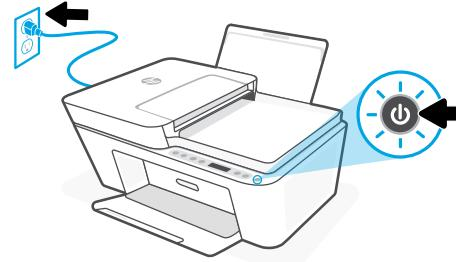
**EN** Plug in and turn on the printer.
