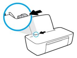
3. Insert one or more envelopes into the far-right side of the input tray and slide the stack of envelopes down until it stops.
