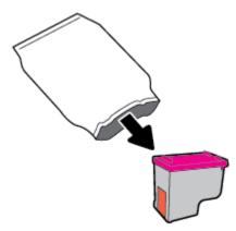
**b.** Remove the plastic tape using the pull tab.
