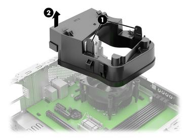
To install the fan shroud, reverse the removal procedures.
