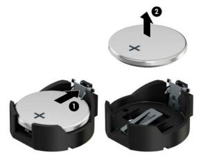
6. To insert the new battery, slide one edge of the replacement battery under the holder's lip with the positive side up (1). Push the other edge down until the clamp snaps over the other edge of the battery (2).
