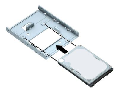
**8.** Secure the drive to the bay adapter bracket by installing four black M3 adapter bracket screws through the underside of the bracket and into the drive.
