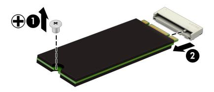
To install the solid-state drive, reverse the removal procedure.
