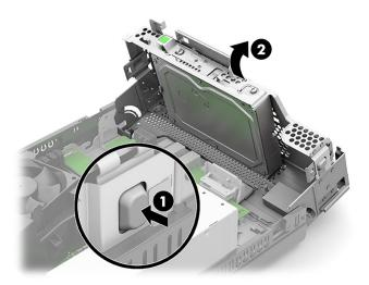
To reset the drive cage, reverse the removal procedure.
