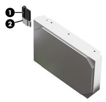
6. To install a new hard drive, you must transfer the silver and blue isolation mounting guide screws from the old hard drive to the new hard drive.
