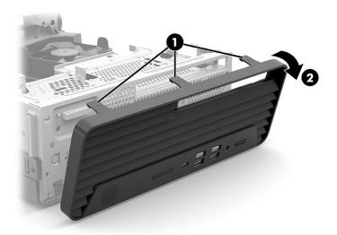
3. Remove the bezel from the access panel.
