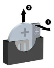
8. Insert the new battery and position the clip back into place.
