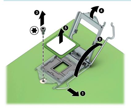
To replace the processor, reverse the removal procedures.
