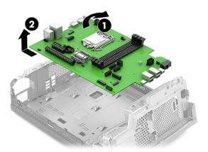
To install the system board, reverse the removal procedures.
