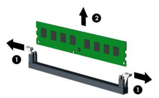
To install a memory module, open both latches of the memory module socket (1), and insert the memory module into the socket (2). Press the module down into the socket so that the module is fully inserted and properly seated. Be sure that the latches are in the closed position (3).
