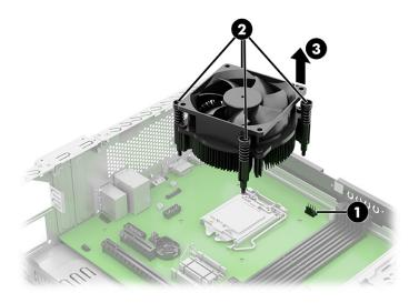
IMPORTANT: Tighten heat sink retaining screws in diagonally opposite pairs (as in an X) to evenly seat the heat sink on the processor to avoid damage that could require replacing the system board.
