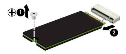
To install the solid-state drive module, reverse the removal procedure.
