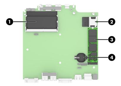
2. To release the battery from its holder, squeeze the metal clamp that extends above one edge of the battery (1). When the battery pops up, lift it out (2).
