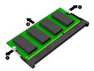
**4.** Slide the new SODIMM into the socket at approximately a 30° angle **(1)**, and then press the SODIMM down **(2)** so that the latches lock it in place.
