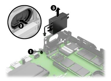
To install the speaker, reverse the removal procedures.
