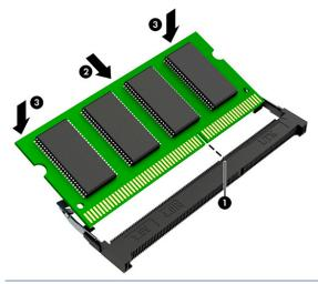
NOTE: A memory module can be installed in only one way. Match the notch on the module with the tab on the memory socket.
