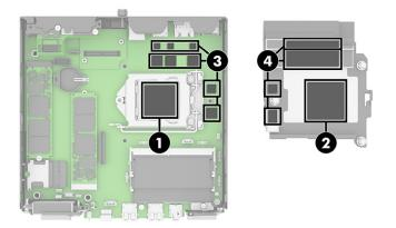
**IMPORTANT:** Tighten heat sink retaining screws in diagonally opposite pairs (as in an X) to evenly seat the heat sink on the processor to avoid damage that could require replacing the system board.
