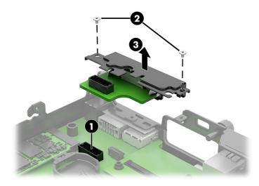
To install flex I/O connector board, reverse the removal procedure.
