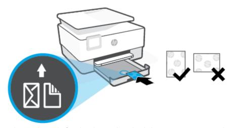
Make sure the stack of card or photo is aligned with the appropriate paper size lines on the front of the tray. Also, make sure the stack of card or photo does not exceed the stack height marking on the left edge of the tray.
