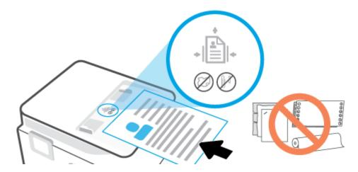
2. Slide the paper-width guides inward until they stop at the left and right edges of the paper.
