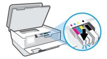
MOTE: Make sure that the color-coded letter on the cartridge matches that on the slot.
