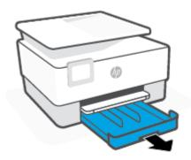
2. Slide the paper-width guides to the edges of the input tray.
