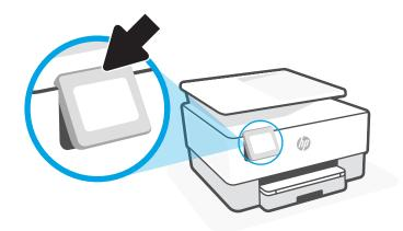
NOTE: Return the control panel to its original position by pushing down the bottom until it is back in place.
