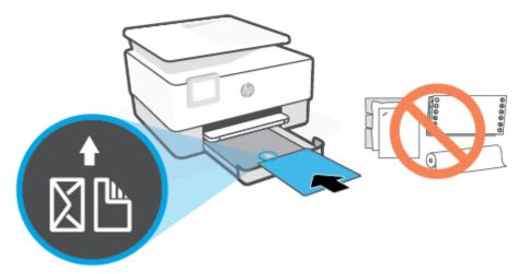
Make sure the stack of paper is aligned with the appropriate paper size lines on the front of the tray. Also, make sure the stack of paper does not exceed the stack height marking on the left edge of the tray.
