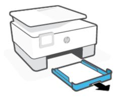
3. Check the input tray area underneath the printer. Removed the jammed paper.
