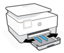
3. Press the button near the front left of the tray to extend the input tray.
