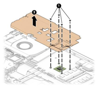
9. Thoroughly clean the thermal material from the surfaces of the heat sink and the system board components each time the heat sink is removed. Replacement thermal material is included with the heat sink and system board spare part kits.
