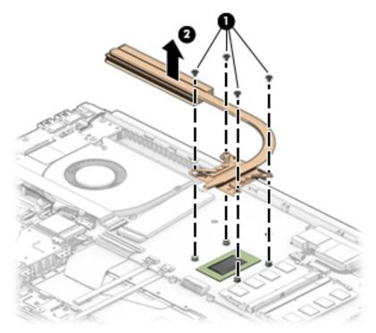
6. Thoroughly clean the thermal material from the surfaces of the heat sink and the system board components each time the heat sink is removed. Replacement thermal material is included with the heat sink and system board spare part kits.
