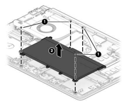
Reverse this procedure to install the battery.
