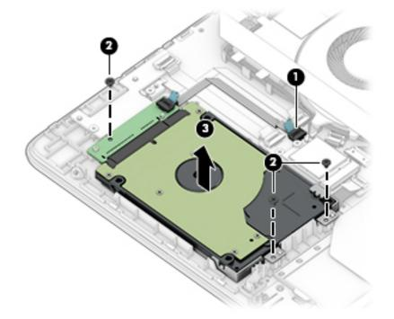
**4.** If it is necessary to remove the bracket from the hard drive, remove the Phillips M3.0 × 3.0 screw **(1)** that secures the bracket to the drive, rotate the bracket away from the drive **(2)**, and then pull the bracket off the drive **(3)**.
