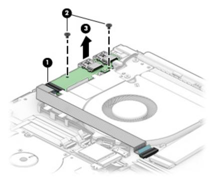
Reverse this procedure to install the USB board.
