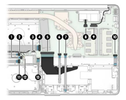
2. Remove the three Phillips M2.0 × 2.8 screws (1) that secure the system board to the computer.
