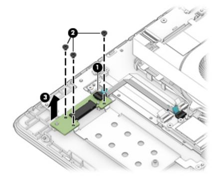
Reverse this procedure to install the solid-state drive board.
