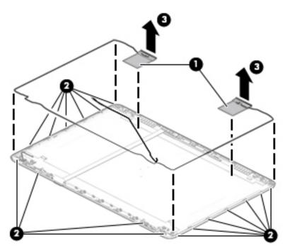
The wireless cables and antennas are available using spare part number L52018-001 for dual antennas or L52017-001 for single antennas..
