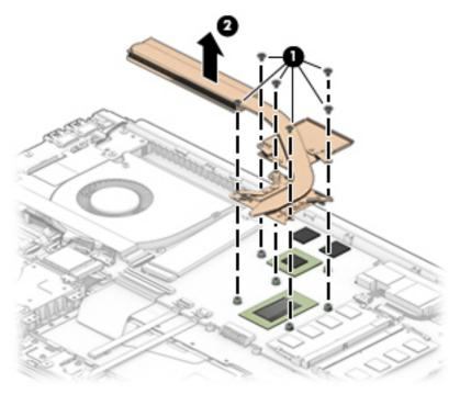
3. Thoroughly clean the thermal material from the surfaces of the heat sink and the system board components each time the heat sink is removed. Replacement thermal material is included with the heat sink and system board spare part kits.
