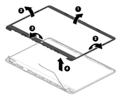
The display bezel is available using spare part number L52014-001.
