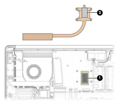
7. **Fanless models:** In the order indicated on the heat sink, remove the four Phillips M2.0 × 2.8 screws (1) that secure the heat sink to the system board.
