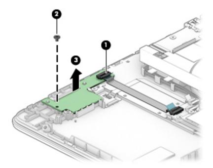
Reverse this procedure to install the card reader board.
