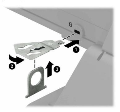
5. Slide the security cable through the security guide installed on the monitor.
