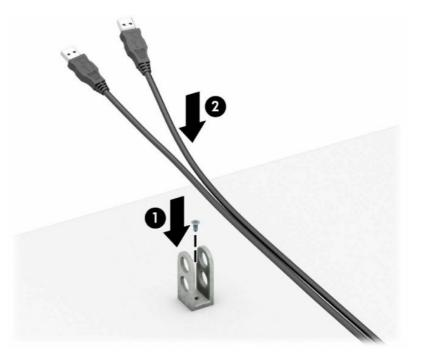
7. Slide the security cable through the holes in the accessory cable fastener.
