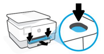
2. Remove the input tray by pulling it all the way out of the printer.
