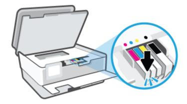
NOTE: Make sure that the color-coded letter on the cartridge matches that on the slot.
