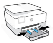
**5.** Reinsert the input tray into the printer.
