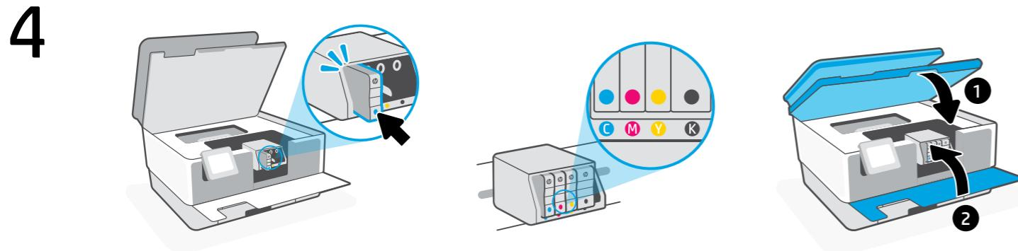
**EN** Insert each cartridge securely into the indicated slot. Close both doors.
