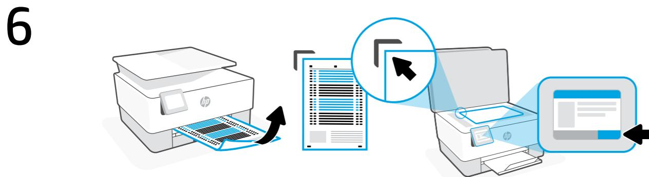
**EN** Use the control panel to print and scan the alignment page.
