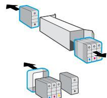
**EN** Open the front door and then lift the cartridge access door by the scanner lid. Unpack cartridges.
