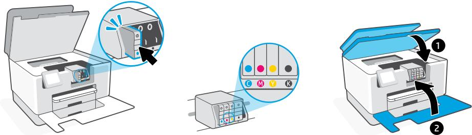
**EN** Insert each cartridge securely into the indicated slot. Close both doors.
