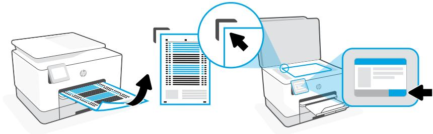
**EN** Use the control panel to print and scan the alignment page.
