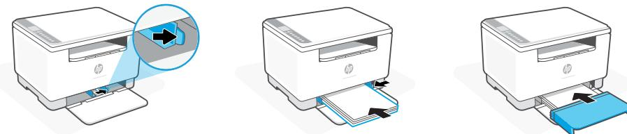
**EN** Slide out the guides. Load Letter or A4 paper and adjust the guides. Slide the tray cover into place.
