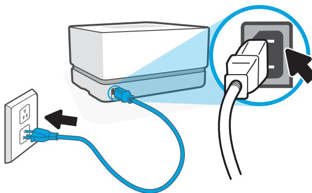
**EN** Plug in the printer. The printer turns on when it is plugged in and can take up to 1 minute to warm up. You will hear a series of noises, which is normal. When the Ready light
