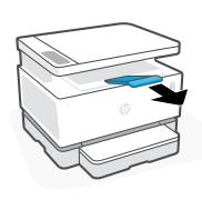
EN Install the input tray, load paper, and then slide the cover into place over the tray. Pull out the output bin extension.
