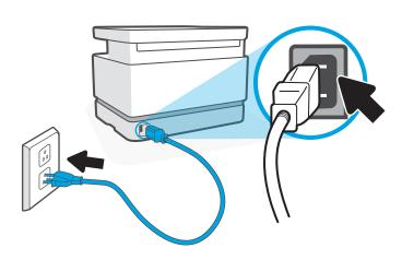
Plug in the printer. The printer turns on when it is plugged in and can take up to 1 minute to warm up. You will hear a series of noises, which is normal. When the Ready light ① stops blinking, the printer is ready.
