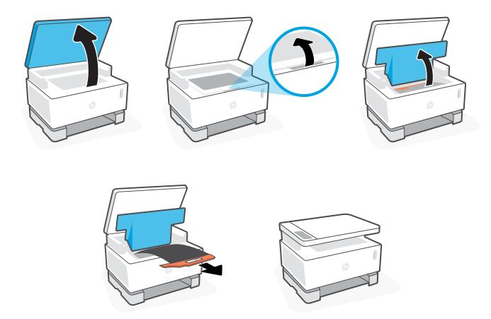
Remove the packing tape. Lift the scanner and the top cover. Remove and recycle the orange plastic handle with the attached black sheet.
