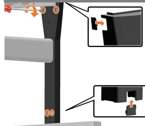
**EN** Insert another set of small covers, then mount the cover at the other side of the stand and fix with 4 PT5x10 screws.
