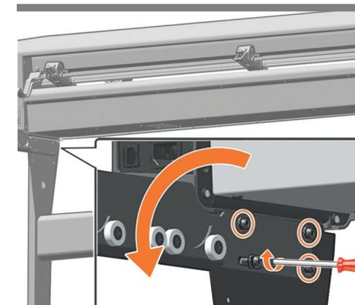
**Mount the left and right roll support brackets and fix with 4 M5x18 screws each side. Use the 3 mm tool. Rotate the left and right plates.**
