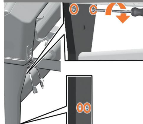
**EN** Guide the cables through the slots in the side cover and fix with 4 PT5x10 screws.
