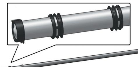
**EN** Slide the two guiding bushes and the brake over a roll as shown. Check the parts are well positioned.
