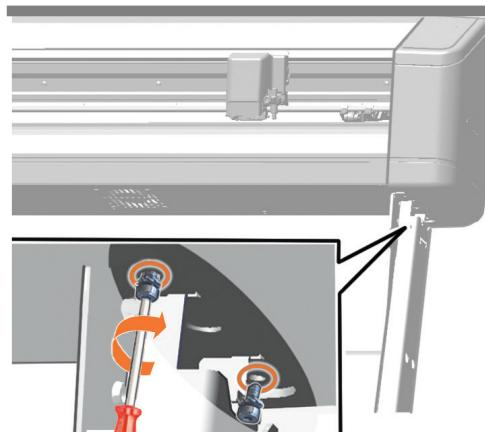
**EN** Fix the cutter to the stand with two M5x18 screws each side.
