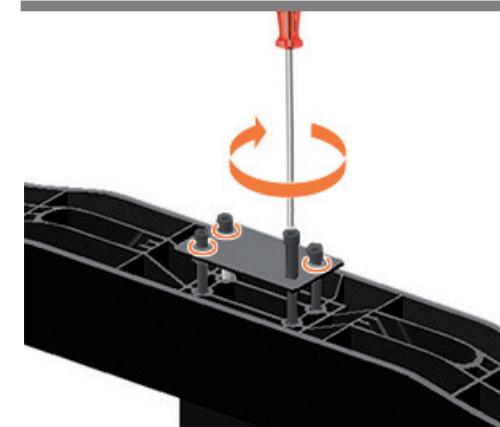
**EN** Mount both feet to the legs with a clamp plate and 4 M5x60 screws and washers each side.
