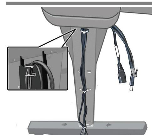
**Optional:** The right-hand side, fix the cable to the stand with 4 cable ties. Align the marks on the cables with the top cable tie.
