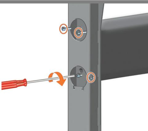
**EN** Firmly insert 2 M5x18 screws and washers just above the two screws that are in the slots at each side.
