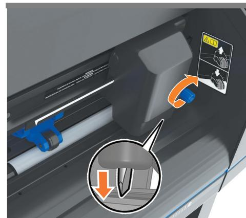
**Important:** If the knife is not installed, take it from the accessory box and install it. If the knife is inserted in the holder, extract it to use the cutter. See the user guide for information on how to use the cutter.
