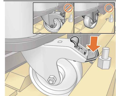
\*Position the 4 wheels in the direction of the ramp, then lock the 2 front wheels.
