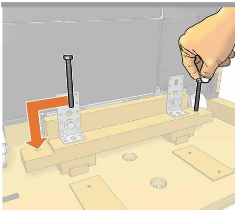
\*Move the carriage bolts to the holes on the sides of the lifter.
