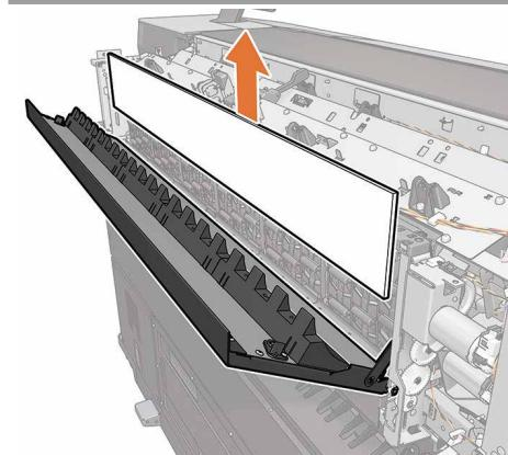
**4000/3900 Printer Series only:** Remove the foam from the stacker door.
