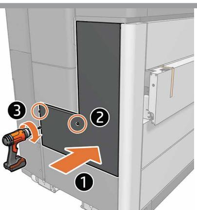
**EN** If an extra drawer is not required; replace the cover and screws, starting with the center screw.
