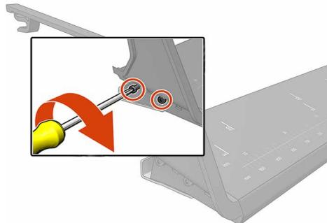
Fix it with 2 screws at each side.
