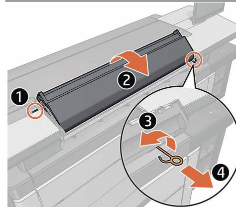
**MFP only:** Pull out the transport lock as far as possible and remove the protective sheet. Open the scanner cover and pull out the transport lock rotating it.
