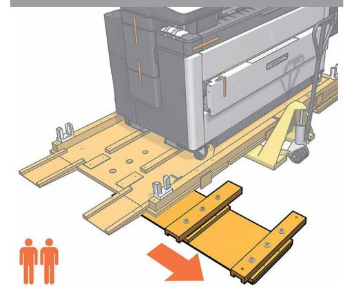
\*Remove the wood block from the on the side you are going to use to lower the printer.
