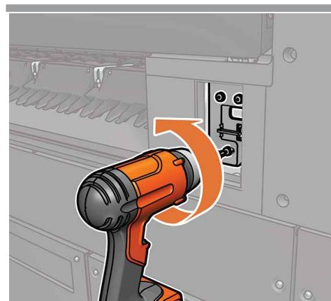
**EN** Remove 3 screws and the two dryer lock plates on the right and left sides.
