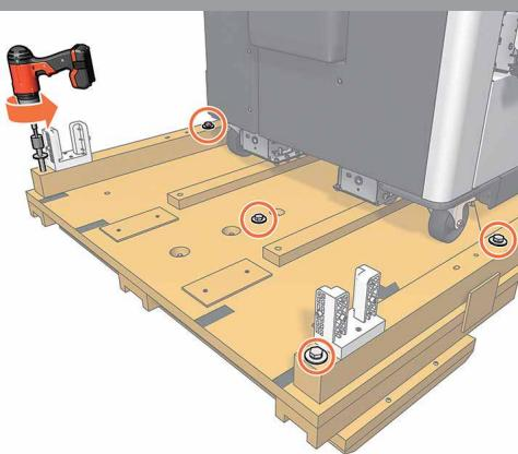
**EN** \*Remove the 5 bolts marked with a black circle on the side you are going to use to lower the printer; use a hammer if required to release them.
