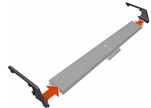
**EN** Place the two end pieces on the loading table.
