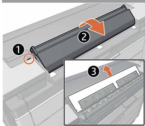
**EN** Open the scanner cover and remove the foam. Gently wipe the glass plate and the surrounding area with a lint-free cloth dampened with water.
