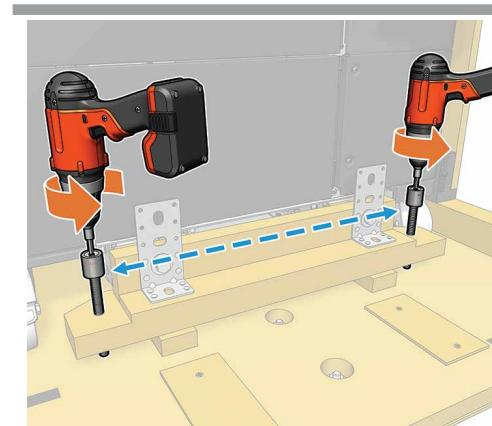
\*Use the carriage bolts to lower the lifter until the printer rests on the wheels, then remove the bolts.
