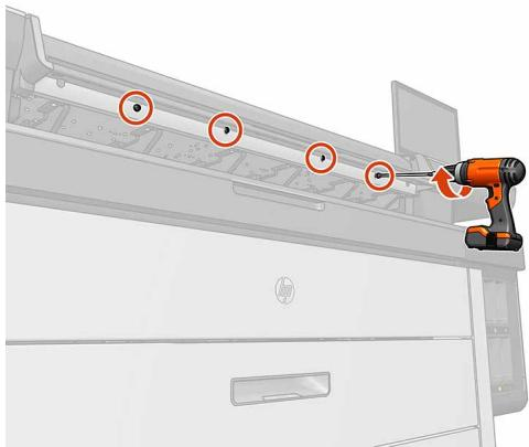
**EN** Fix using 4 screws with washers.
