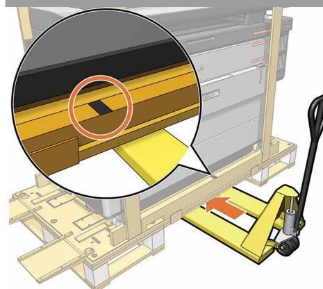
\*Place the forklift under the pallet where marked, and raise the printer.
