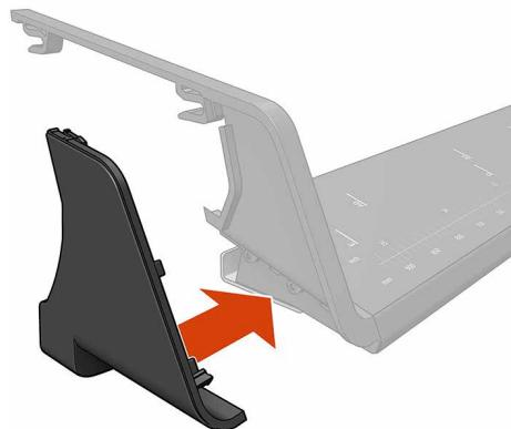
Assemble the end pieces by clipping the 2 parts together.
