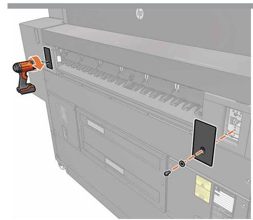
**EN** If planning to install any output accessories, install the hooks (found in the accessory box), or the covers if not installing any.
