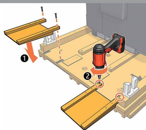
\*Fix the ramps found in the accessory box on the side you are going to use to lower the printer.
