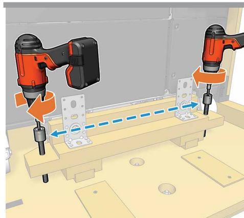
\*Screw in the carriage bolts to lift the lifter. Lift slightly on each side and repeat.
