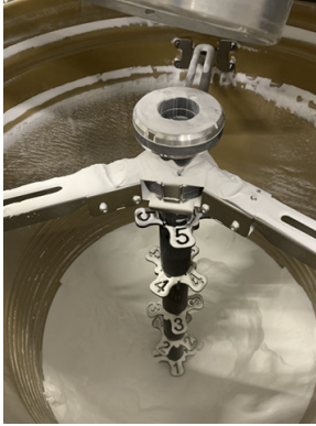
Figure 6-1 The numbers in the external tank indicate the material level.
