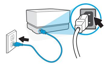
Plug in the printer. The printer turns on when it is plugged in and can take up to 1 minute to warm up. You will hear a series of noises, which is normal. When the Ready light  $\odot$  stops blinking, the printer is ready.
