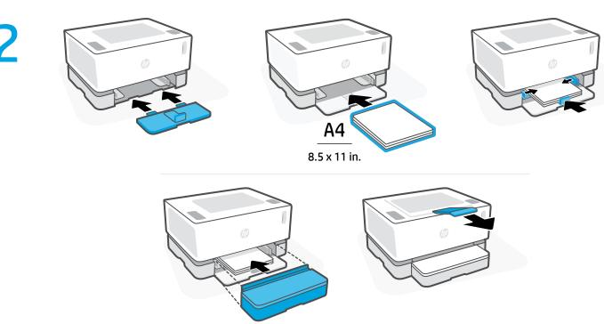
Install the input tray, load paper, and then slide the cover into place over the tray. Pull out the output bin extension.
