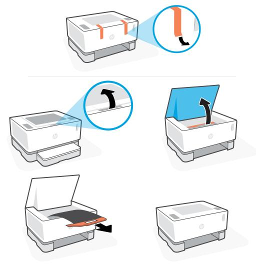
Remove the packing tape. Lift the top cover, and then remove and recycle the orange plastic handle with the attached black sheet.
