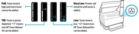
Toner can be added when the **Reload Status** light : next to the reload port glows white. Toner cannot be added when the light is off. To learn how to add toner, follow the instructions on the HP Toner Reload Kit or download the User Guide from **www.hp.com/support/Neverstop1200**.
