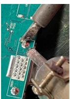
VGA (D-Sub) connector repairing
