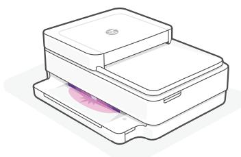
**EN** Plug in to automatically power on. Wait until the printer lighting is purple and continue to step 3.
