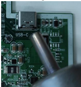
Remove USB-C connector
