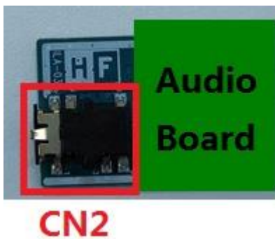
Audio Board showing location of connector
