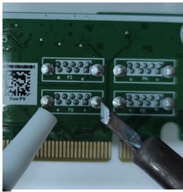
Remove USB connectors
