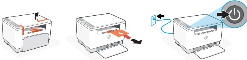
**EN** Remove all tape and pull the paper sheet from the printer. Plug in and turn on the printer.
