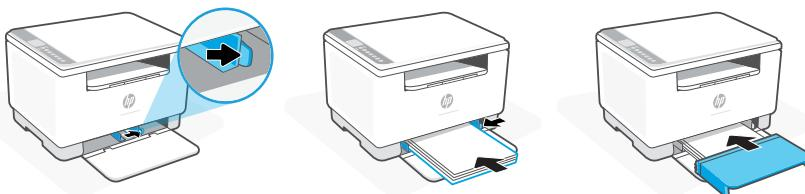
**EN** Slide out the guides. Load Letter or A4 paper and adjust the guides. Slide the tray cover into place.
