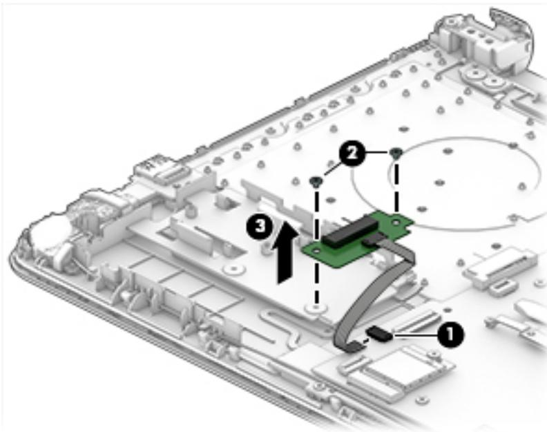
Reverse this procedure to install the solid-state drive board and cable.
