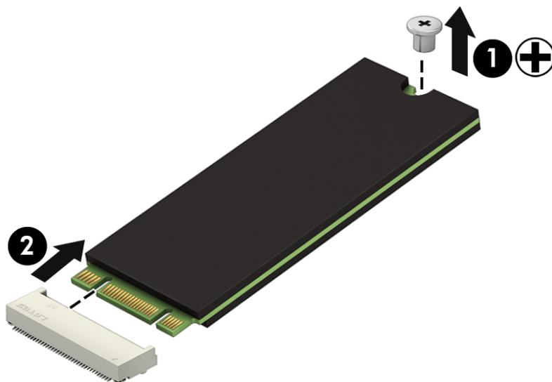
Reverse this procedure to reassemble and install the solid-state drive.
