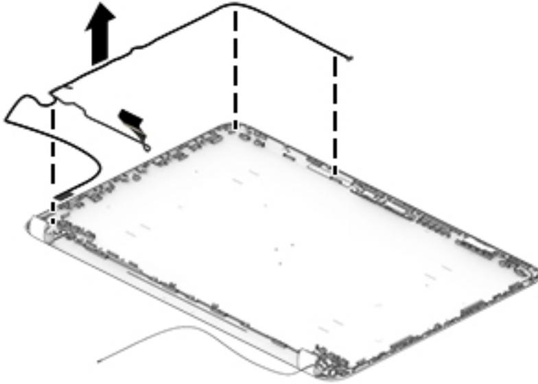
7. If replacing the display enclosure, be sure that the subcomponents (including the webcam/microphone module, the antenna receivers, and all associated cables and hardware) are transferred to the new enclosure.
