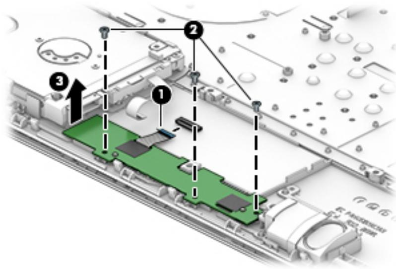
Reverse this procedure to install the TouchPad button board and cables.
