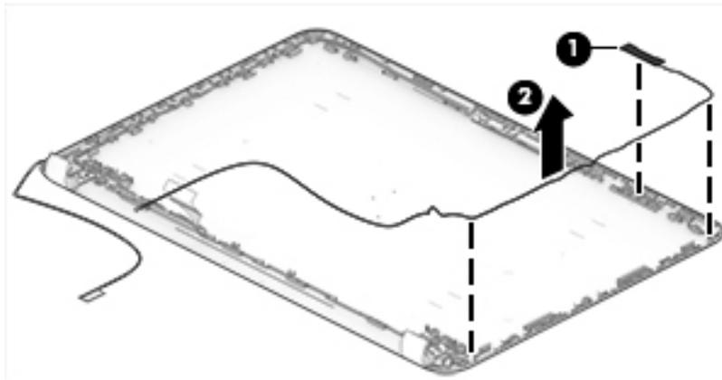
6. To remove the display/webcam cable, remove the cable from the clips built into the display enclosure, and then remove the cable from the display enclosure.
