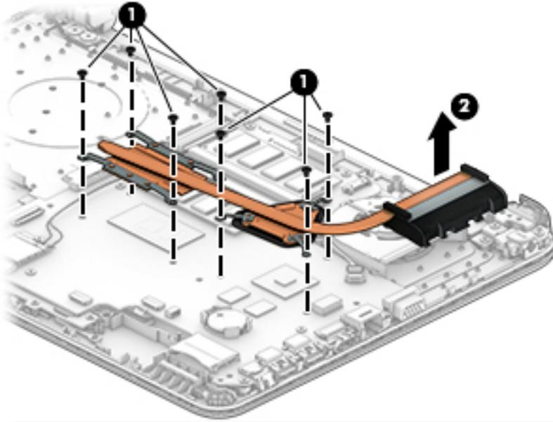
4. On models with UMA graphics, remove the four Phillips PM2.0×3.0 screws (1) on the heat sink that secure the heat sink assembly to the system board.
