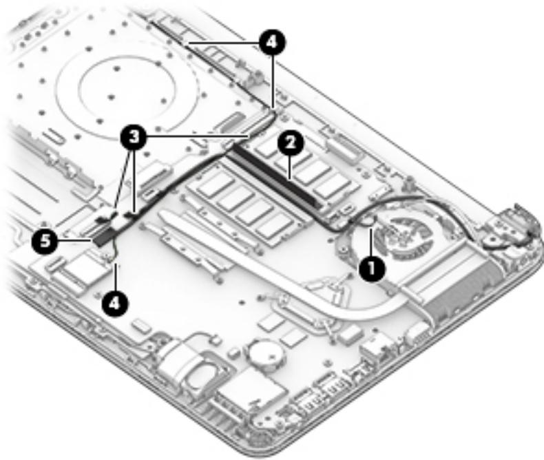
6. Position the computer upright, and then disconnect the following cables from the system board:
