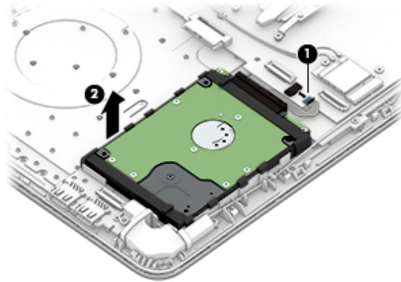
3. To disassemble the hard drive, pull the connector away from the drive to remove it (1).
