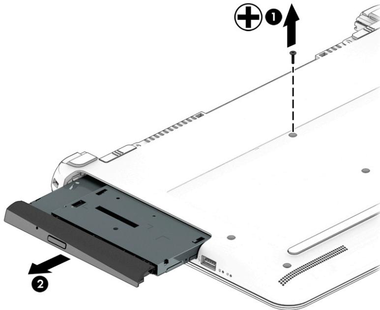
Reverse this procedure to reassemble and install the optical drive.
