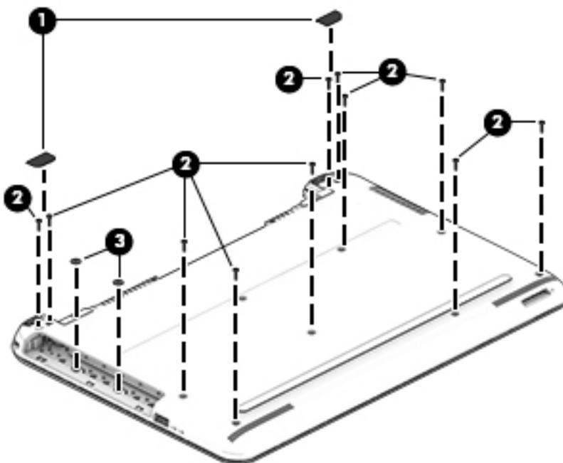
5. Start prying near the optical drive bay and work around to the back and side to separate the bottom cover from the computer **(1)**.
