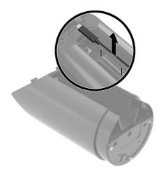
8. Remove the I/O blank from the stand. Replace the access door.
