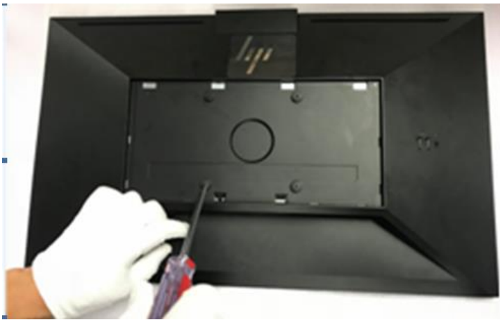
Remove the VESA-screws
