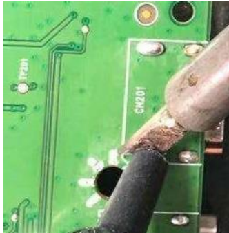
Remove USB connector
