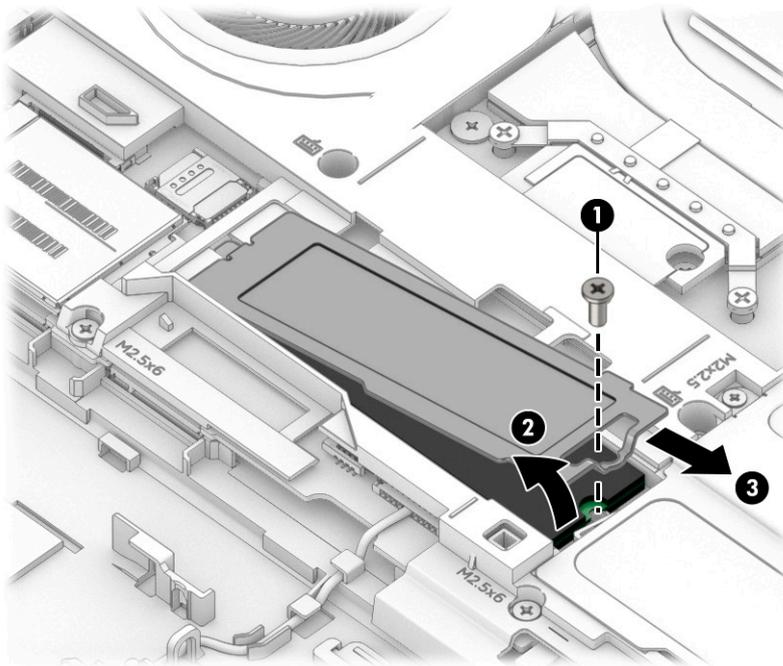
4. Pull the drive away from the socket to remove it (1).
