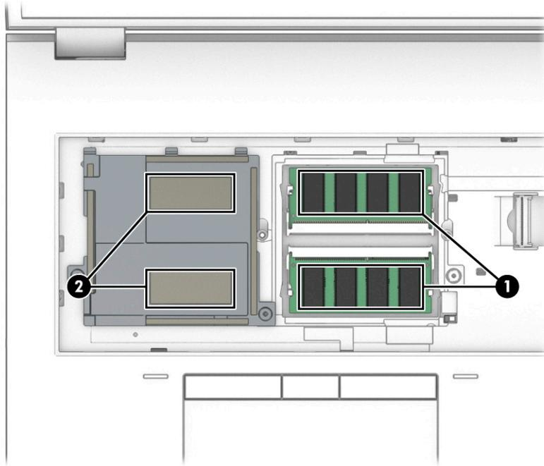
4. Spread the two retention clips outward (1) until the memory module tilts up at a 45° angle, and then remove the module (2). Use the same procedure to remove all memory modules.
