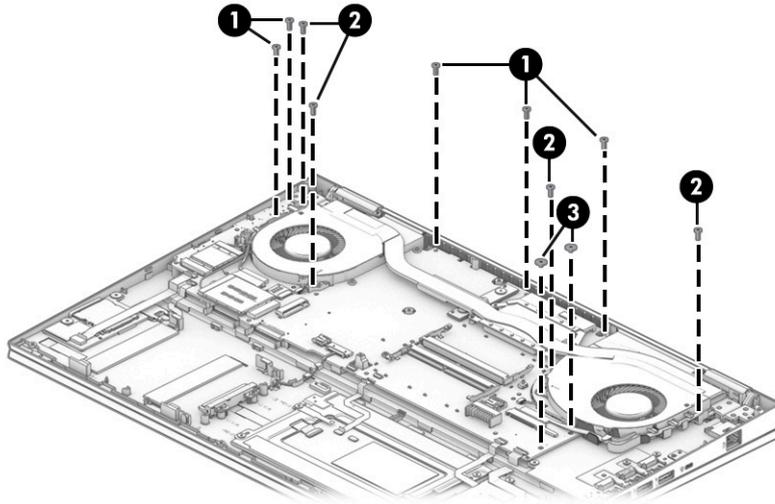
16. Lift the front/right edge of the system board (1) until it rests at an angle.
