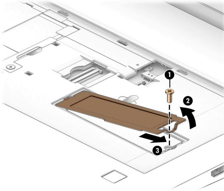
4. A thermal pad services solid-state drive 1 and is located on the solid-state drive cover. Inspect this pad each time the cover is removed. This pad is intended to be reused if it is not damaged. If this pad is damaged and any residue remains on the solid-state drive (1) or the cover (2), thoroughly remove and replace it. If protective releasing paper is attached to the thermal pad, remove it prior to replacement.
