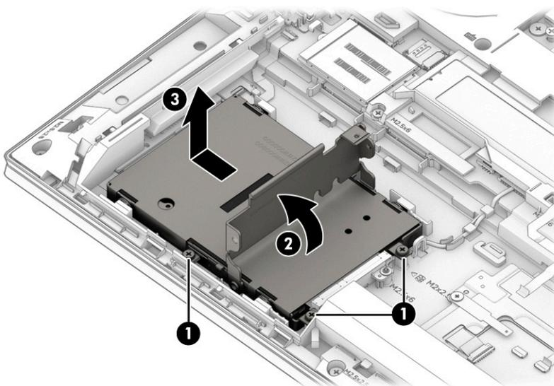
Reverse this procedure to install the hard drive.
