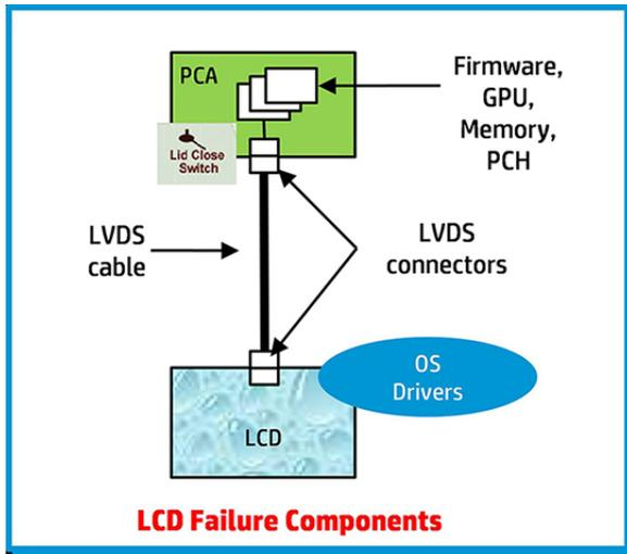
**NOTE:** The lid close switch is a Hall-effect sensor located in the top cover. When the display is closed, the sensor acts like a switch is closed. A notebook can force a video output to an external monitor, or go to hibernation or standby mode through power management. If the display screen does not light up when the display is open, the lid close switch (Hall-effect sensor) could be faulty.
