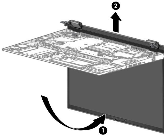
10. If it is necessary to replace the display bezel or the display assembly subcomponents:
