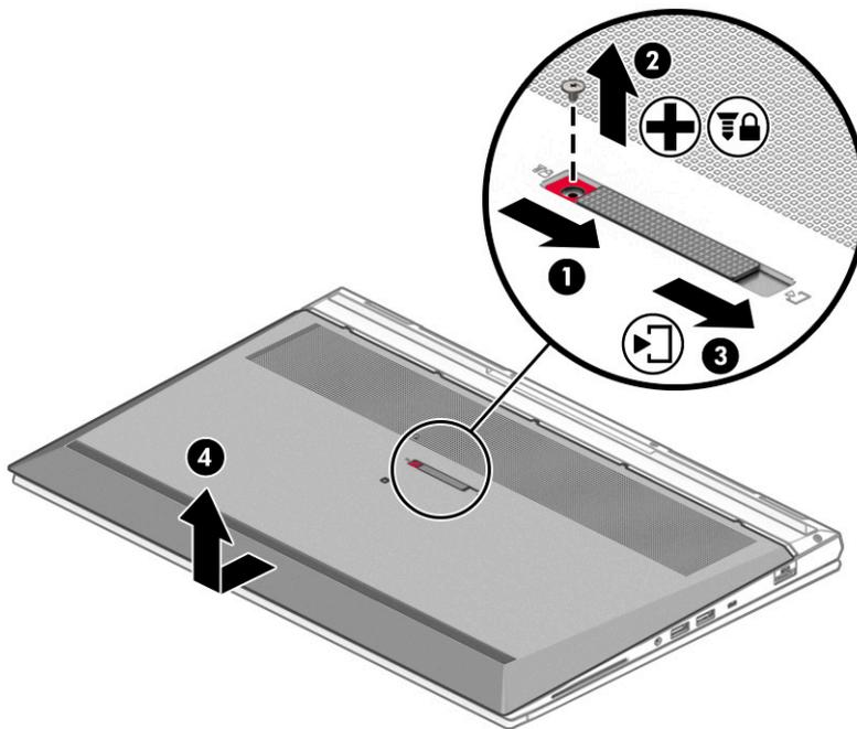
To replace the service cover, reverse the removal procedures.
