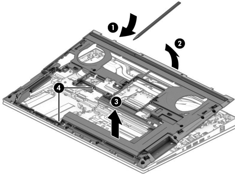
Reverse this procedure to install the bottom case.
