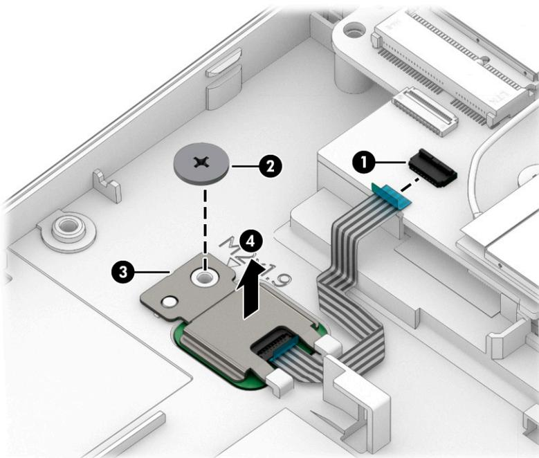
Reverse this procedure to install the fingerprint reader module and cable.
