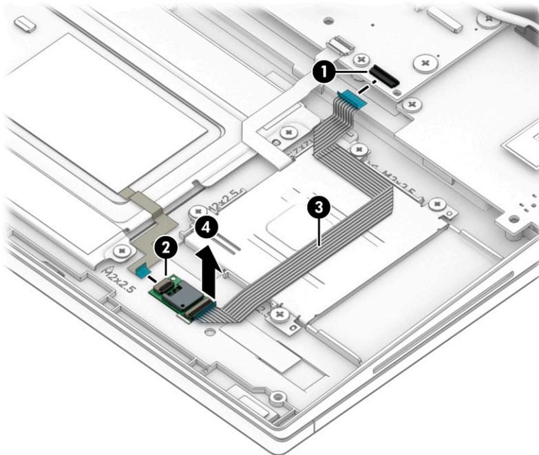
Reverse this procedure to install the NFC module and cable.
