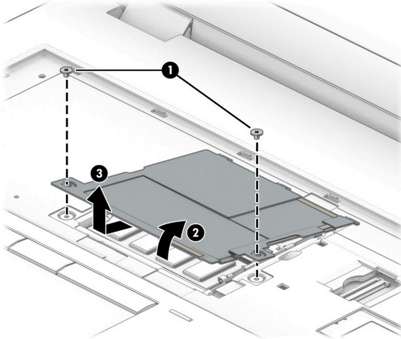
Thermal pads service memory modules 1 and 3 and are located on the memory module compartment cover. Inspect these pads each time that the cover is removed. These pads are intended to be reused if they are not damaged. If these pads are damaged and any residue remains on the memory modules **(1)** or the cover **(2)**, thoroughly remove and replace them. If protective releasing paper is attached to the thermal pads, remove it prior to replacement.
