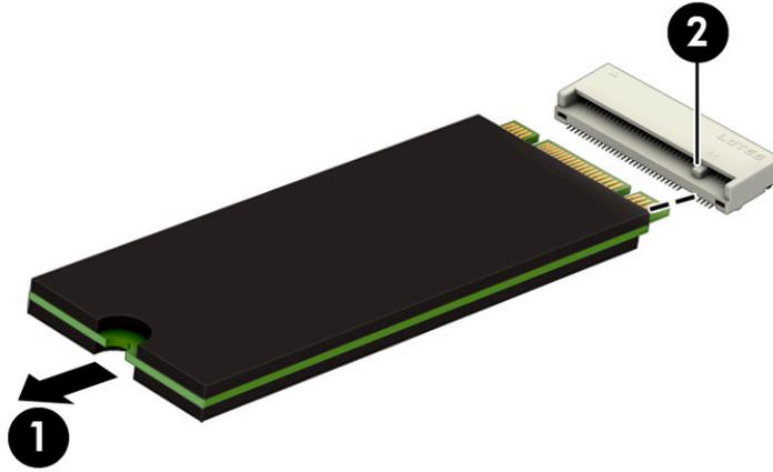
To install the solid-state drive, reverse the removal procedures.
