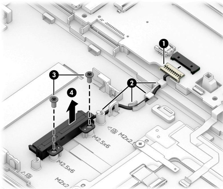
Reverse this procedure to install the hard drive cable.
