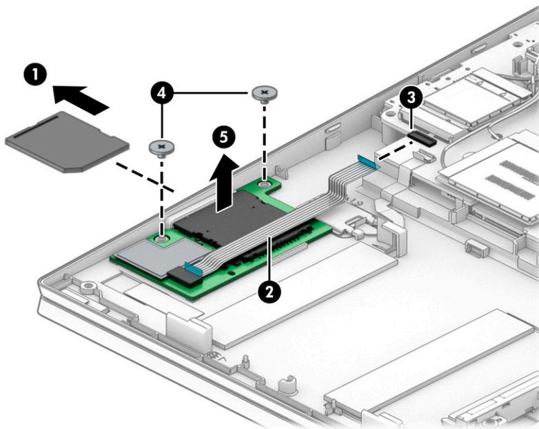
Reverse this procedure to install the SD card board and cable.
