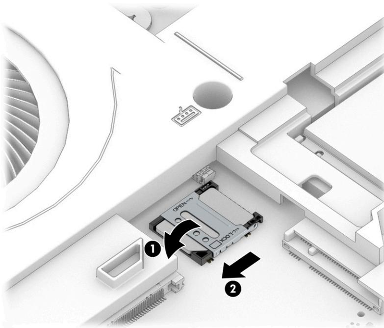
To remove the SIM card, reverse the procedures as described above.
