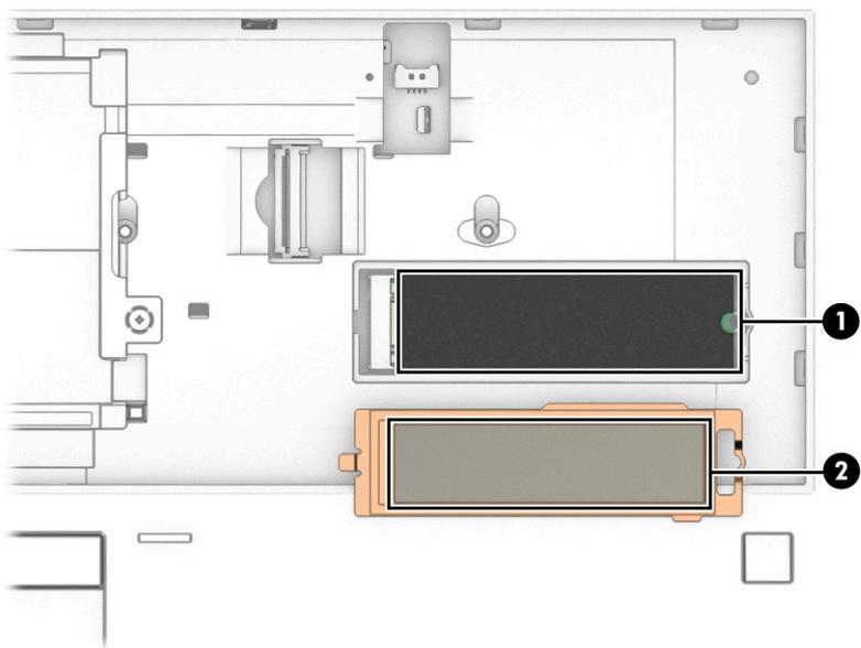
5. Pull the drive away from the socket to remove it (1).
