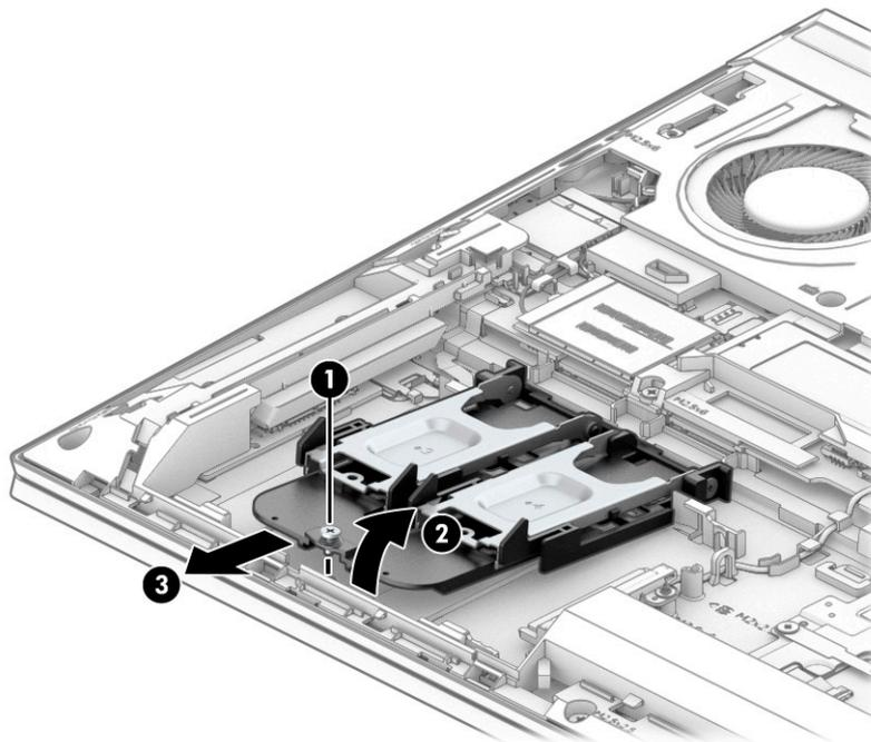
Reverse this procedure to install solid-state drives 3 and 4 and the solid-state drive carrier.
