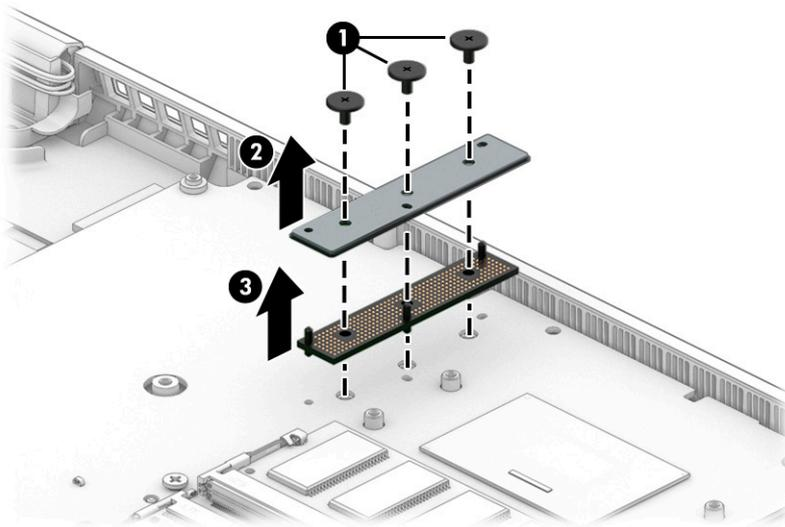
4. Align the pins on the replacement beam connector with the holes in the system board, and then carefully install the beam connector (1) onto the socket on the system board.
