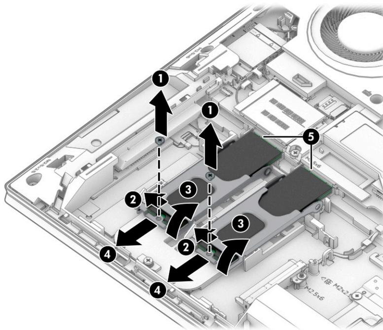
5. If it is necessary to remove the solid-state drive carrier, loosen the captive Phillips screw **(1)** that secures the carrier to the computer.
