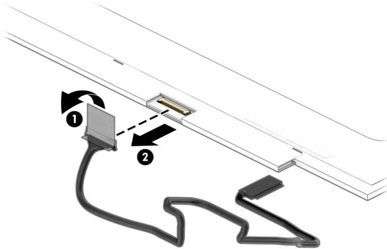
14. If it is necessary to replace the ambient light sensor module:
