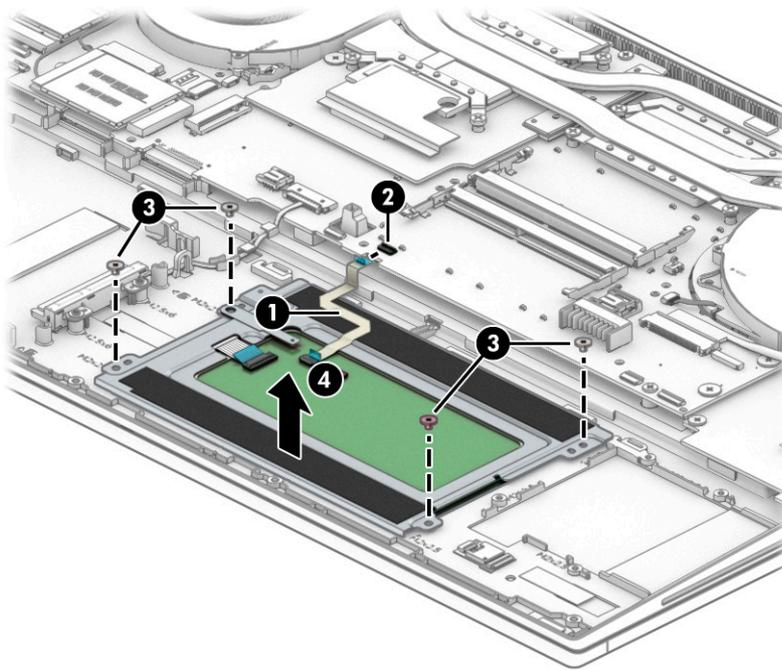
Reverse this procedure to install the touchpad and cable.
