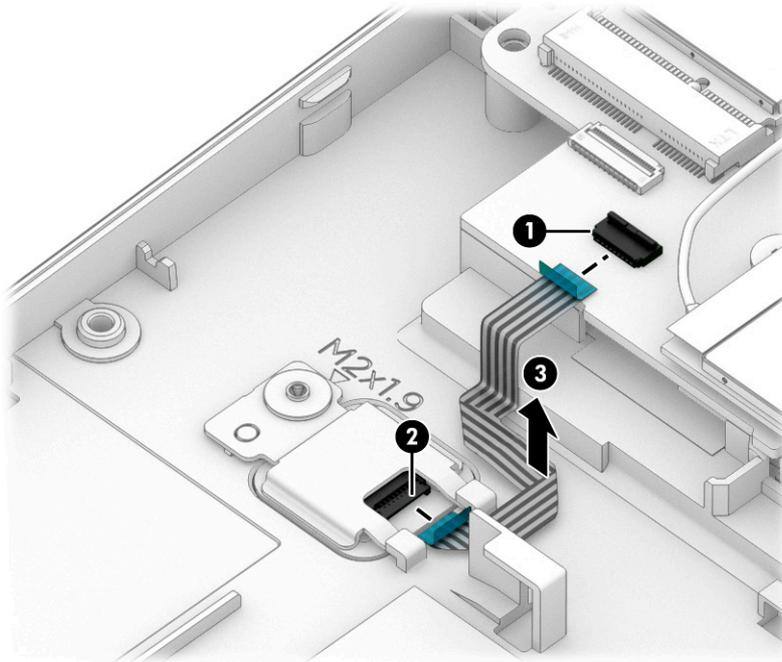
Reverse this procedure to install the fingerprint reader module cable.
