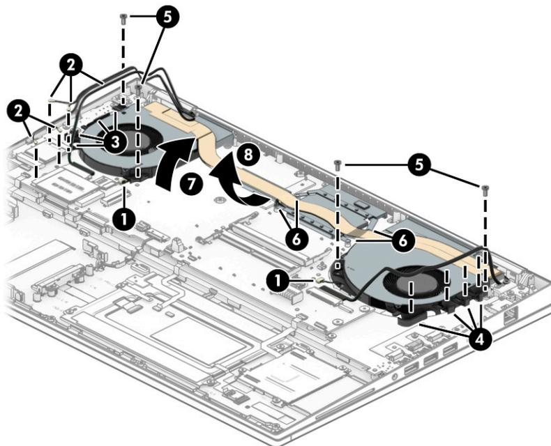
8. Thoroughly clean the thermal material from the surfaces of the fan/heat sink assembly and the system board components each time the fan/heat sink assembly is removed. Replacement thermal material is included with the fan/heat sink assembly and system board spare part kits. The following illustrations show the replacement thermal material locations.
