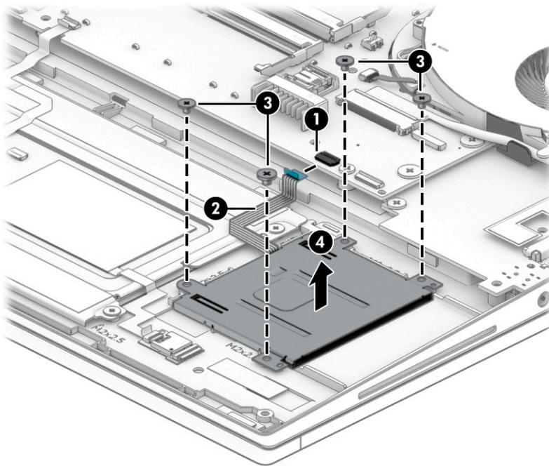
Reverse this procedure to install the card reader board and cable.
