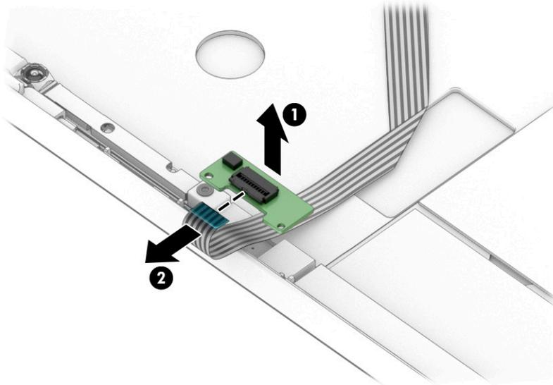
15. If it is necessary to replace the webcam/microphone module and cable:
