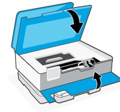
**EN** Remove all packaging and tape. Open the front door and cartridge access door. Remove cardboard. Make sure to close the doors.
