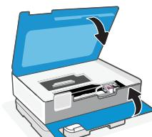
4. Close the carriage access door and front door when finished.
