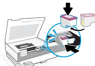
3. Rotate the cartridges so the taller end faces towards the printer. Insert the cartridges and click into place.
