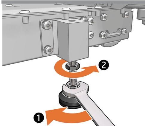
**EN** Level the printer adjusting the height of each foot.
