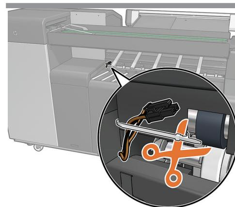
On the left side of the roller tray, remove the cable tie from the power cable.
