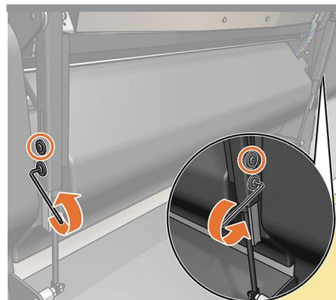
**EN** Pull the folder tray up and loosen the gas springs stoppers.
