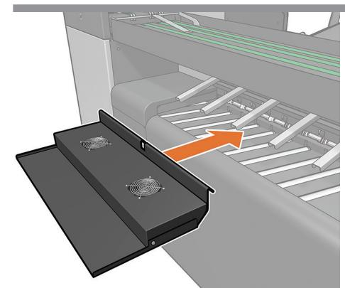
Place the fan unit on the top of the transport tray.
