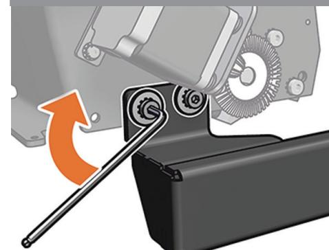
Loosen the screws from the hook, but do not remove them. Push the tray down and then tighten the screw again. Then replace all covers.
