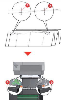
If the misalignment appears on the left, the folder needs to be closer to the right; loosen the two hooks' screws, move the hook, and tighten later.
