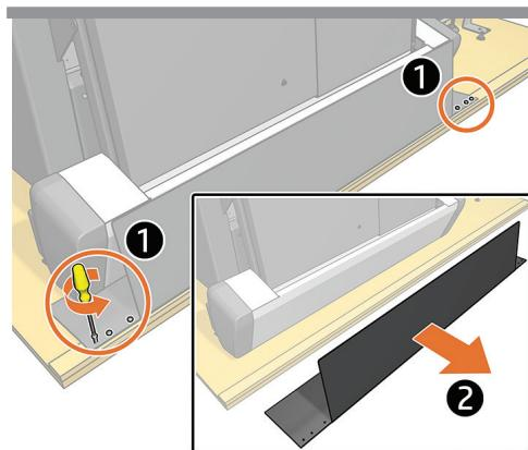
**EN** Remove the 6 torx 30 screws and the bridge protector.
