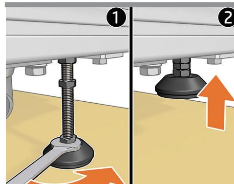
Adjust the levelling pads until the 4 wheels sit correctly.
