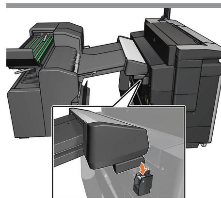
**EN** Connect the folder tray over the printer's hooks.
