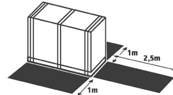
**EN** The space required for assembly is 2,5m (8,2 feet) at the front and 1m (3,3 feet) on each side.
