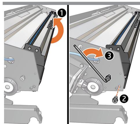
Move the front module so the bottom screw can be fixed with 1 screw on each side in the neighboring hole shown in the image. Screw in on both sides, and tighten the upper screw.
