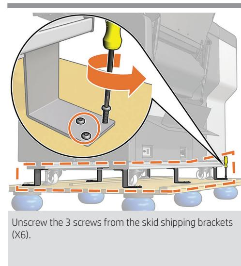
**EN** Unscrew the 3 screws from the skid shipping brackets (X6).
