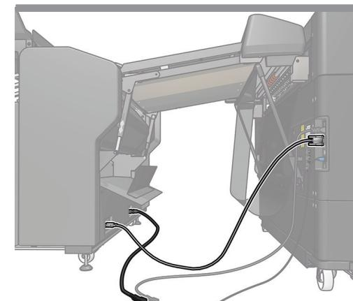
Switch off the printer with the rear button, connect 1 cable from the folder to the printer and another from the folder to the electricity supply.
