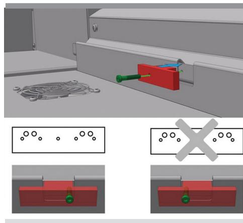
**EN** Assemble the fan unit into the upper and lower support rails. The screw has to be in the fan unit gap.
