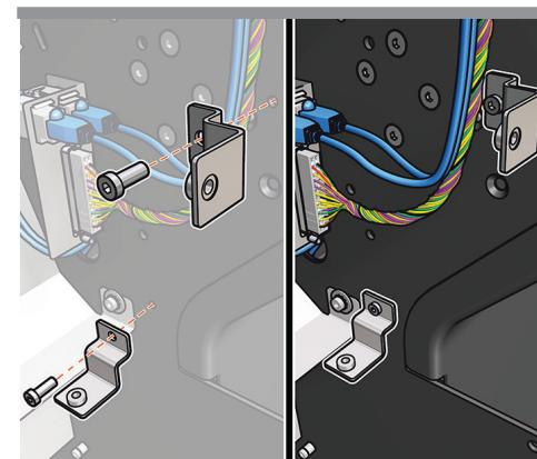
**EN** Place 2 brackets on the right, with one screw on each.
