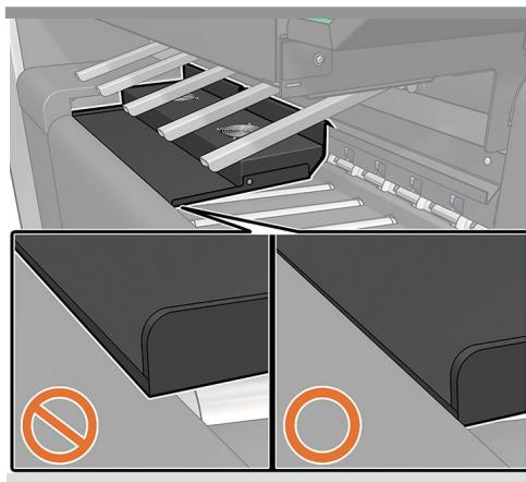
**EN** Please ensure that the fan unit is assembled correctly.
