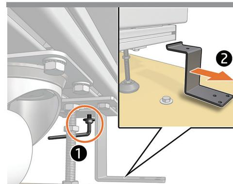
Remove the screw from the top of each bracket and remove the brackets.
