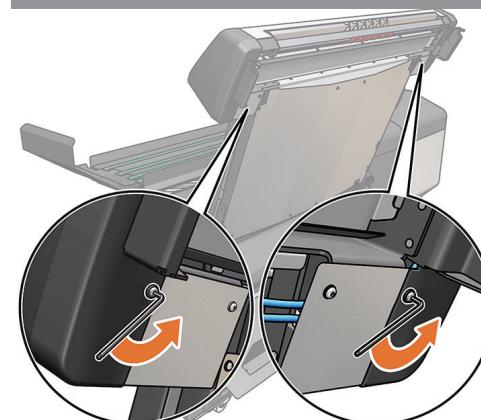
**EN** Remove 1 screw from each side, then remove the piece shown.
