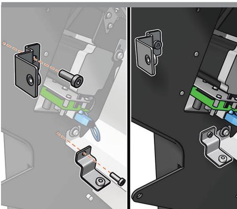
**EN** Place 2 brackets on the left, with one screw on each.
