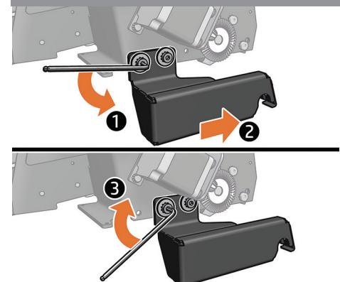
**EN** Remove 2 screws, move the hook upwards, and fix in the 2 front holes.
