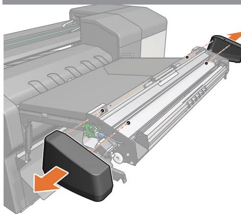
**EN** Remove 2 screws from each side of the folder tray to remove the lateral covers.
