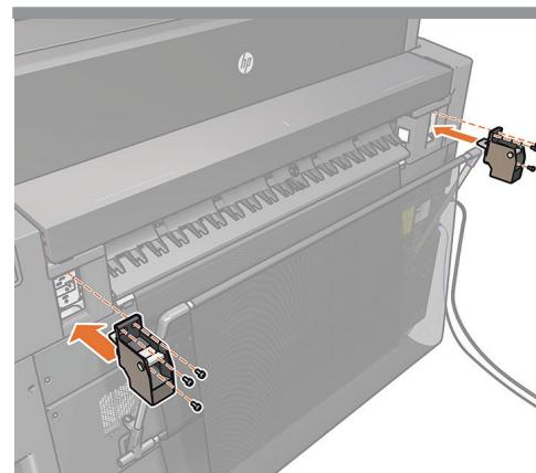
Fix the 2 accessory hooks to the printer with 3 screws each side.
