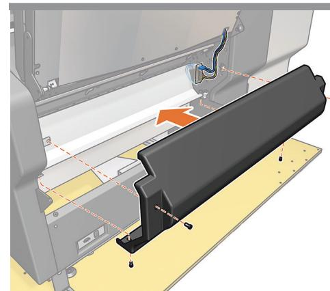
Place bottom cover, and fix it to the brackets with 4 screws.
