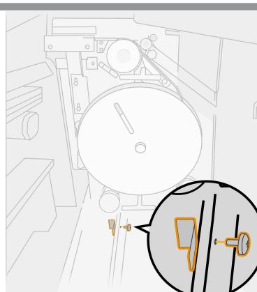
**EN** Remove the piece shown by removing 1 screw on the lateral.
