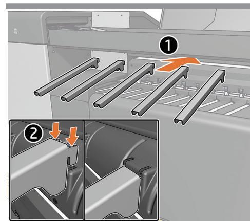
**EN** Place 5 stacker-exit-sliders under the cross-fold tray.
