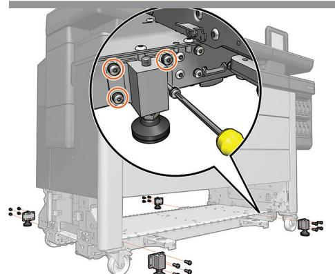
**EN** Fix the 4 levelling feet to the structure base with 4 M6x25 screws each.
