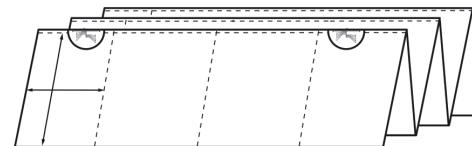
From the front panel (**Internal prints > Output destination prints > Print test on folder to check alignment**) print the test plot to check it is correctly adjusted. Unfold the test plot and check it is folded on the same line. If the plot is not correctly aligned, proceed with steps 55 or 56.
