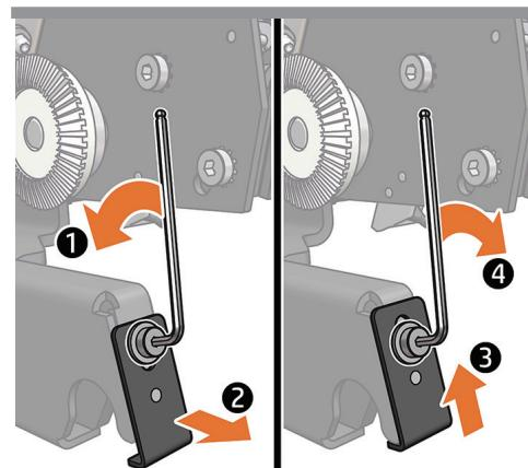
Unscrew the metallic piece on both sides from the extreme of the folder tray and position the pin using the bottom hole.
