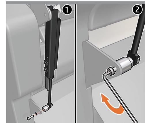
Fix the bottom of the gas spring with 1 screw making sure it is fully tightened. Do the same on the other side.
