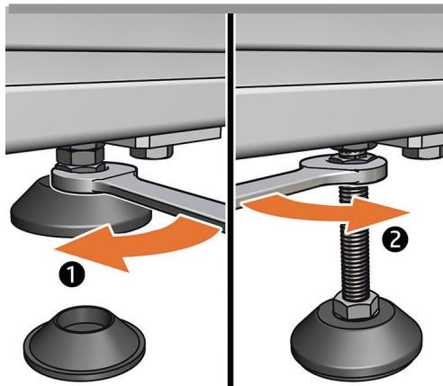
**EN** Adjust the levelling pads to the lowest position. Place the plastic taps under them. Make sure the folder is level and parallel to the printer, making sure to adjust it for any floor unevenness.
