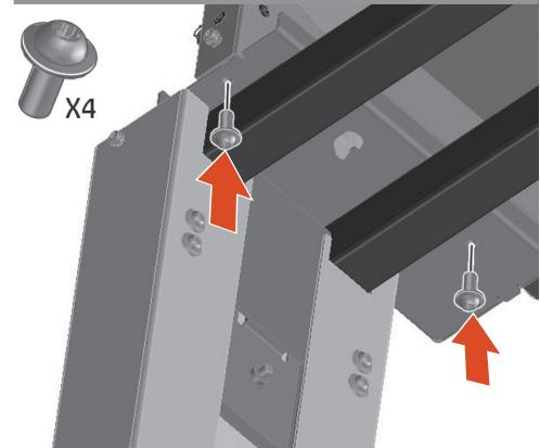
**EN** Fix the chassis to the stand with 2 screws on each side.
