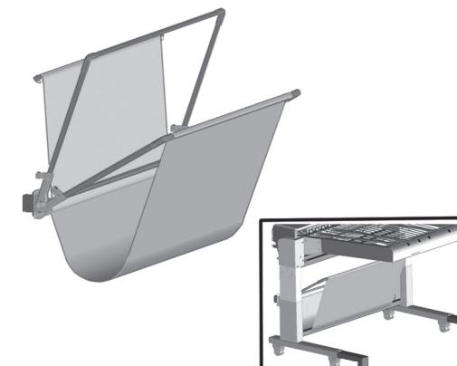
If a basket is attached to the printer; rotate it downwards.
