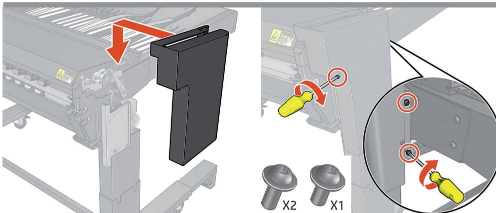
**EN** Install the right-hand side lateral cover, and fix in place with 2xM6 and 1xM4 screws.
