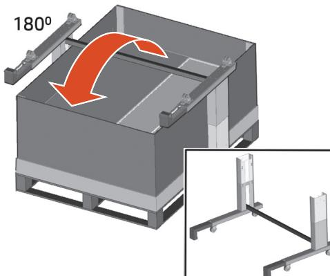
**EN** Remove the corner and rotate the stand base into the upright position.
