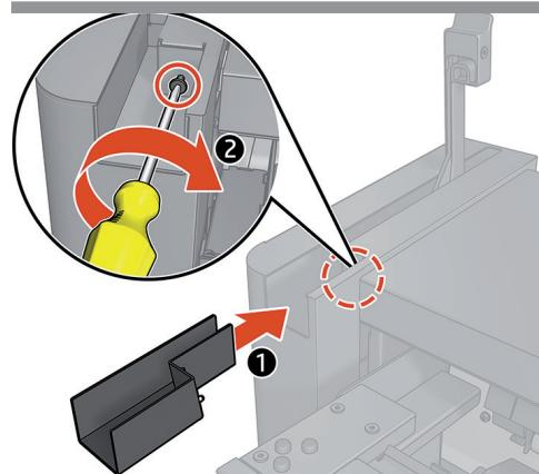
**EN** Install the lever bezel and fix it with 1xM4 screw.
