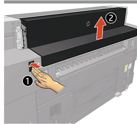
With the printer turned off, open the output module on the back.
