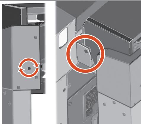
Make sure the latches click into place on both sides, then manually turn the adjustment screws clockwise until resistance is felt.
