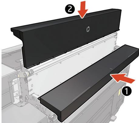
**EN** Install the output module covers starting with the lower one first.
