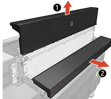
**EN** Remove the 2 output module covers starting with the upper one.
