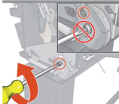
At the right-hand side, remove the screw that blocks the pulley.
