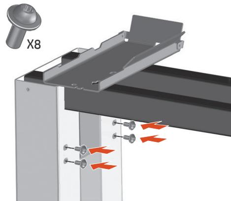
**EN** Fix the top crossbar with 4 screws on the inner part of each side.
