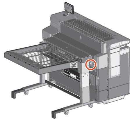
**EN** Make sure the front lateral stacker latches face the printer using the top central marks found on both for reference.
