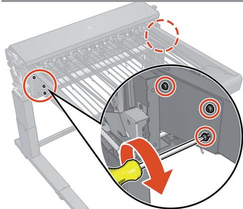
**EN** Fix the tray with 3 screws on each side.
