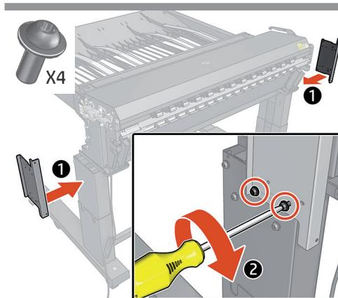
**EN** Install a cover support on both sides, and fix with 2 screws each.
