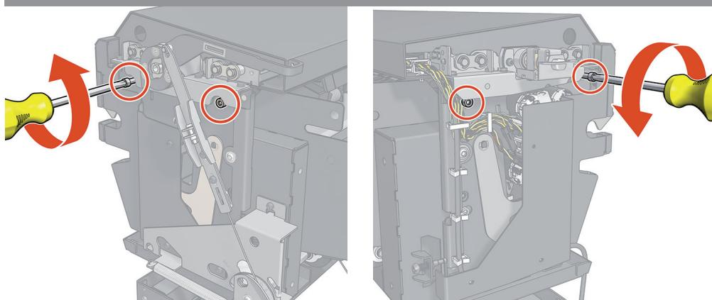
**EN** Remove the 4 screws at the sides that lock the roof (2 screws each side).
