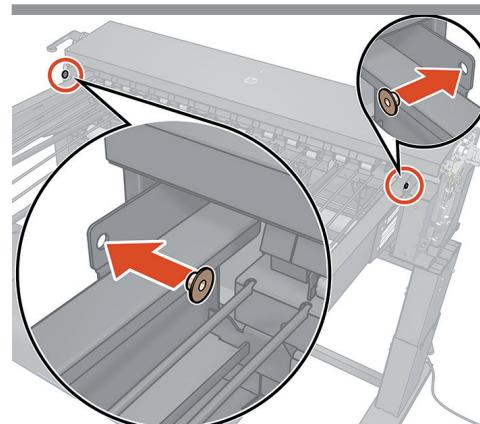
**EN** Insert 2 accessory roof bushings in each side of the tray support.
