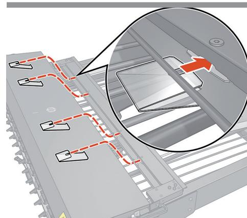
Insert the bottom deflector through the beam hole, and fix it onto the top of the front deflector.
