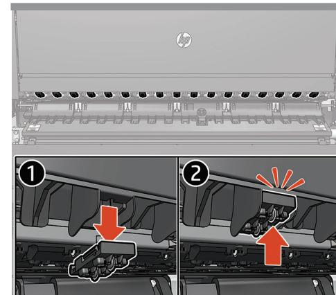
**EN** Only for printer with a top stacker installed: Remove the 17 plastic parts and install the new ones provided.
