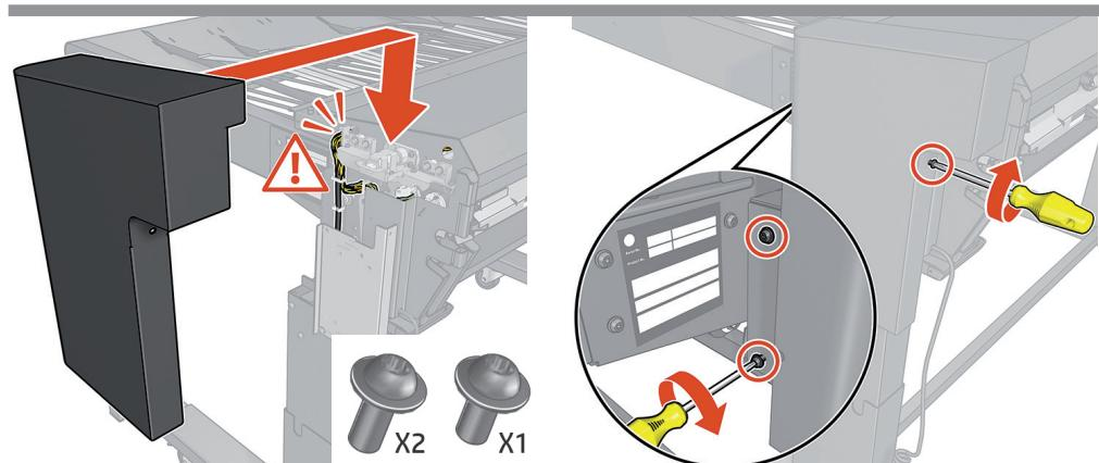
**EN** Install the left-hand side lateral cover, and fix in place with 2xM6 and 1xM4 screws.
