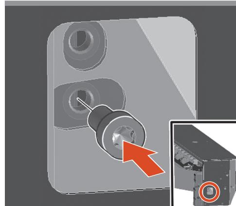
Insert the screws from the previous step into the lower holes.
