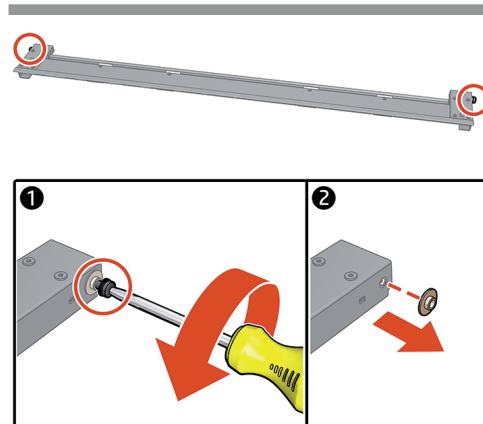
**EN** Remove the screws and bushing from each side of roof beam.
