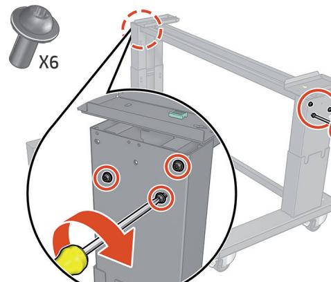
**EN** Fix the crossbar to the stand base with 3 screws on the external part of each side.
