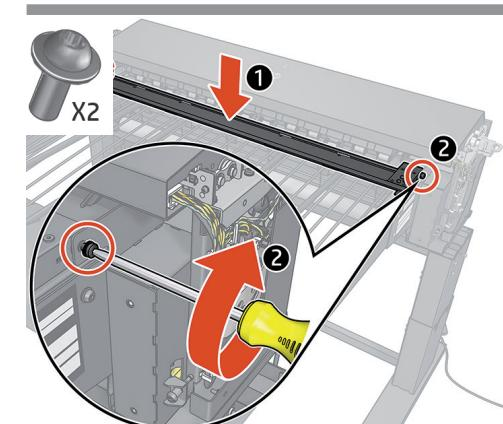
**EN** Place the accessory roof on top of the stacker tray and align the bushing holes. Fix it in place with the 2 screws.
