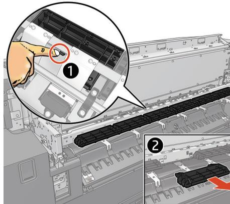
**EN** Remove the plastic pieces; there is a tab in the inner part, pull it down in order to easily remove the pieces. The tabs can then be discarded.
