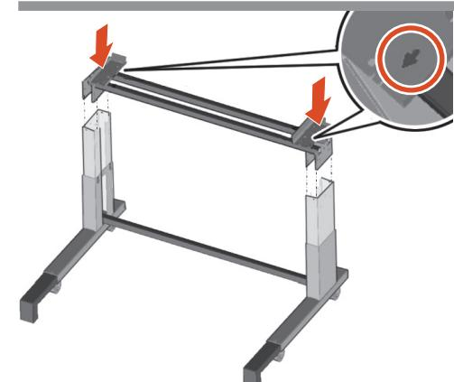
Place the crossbar onto the top of the stand base, making sure both arrows are as indicated; the arrows should point towards the long part of the leg.
