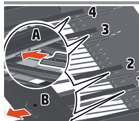
Remove the plastic protectors and tapes. Insert the 4 deflectors into position (A). Push them until the deflector is seen at the opposite side of the beam(B) and you hear a click.
