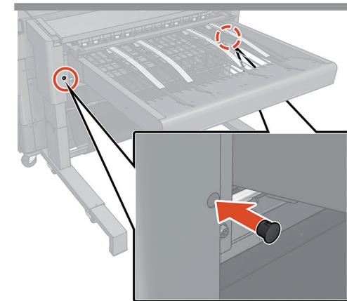
Put the plugs into the covers at both sides.
