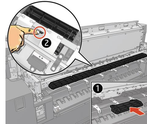
**EN** Insert the 6 new brackets provided into position where the discarded brackets were placed (1). Make sure the brackets are fully in place (2).
