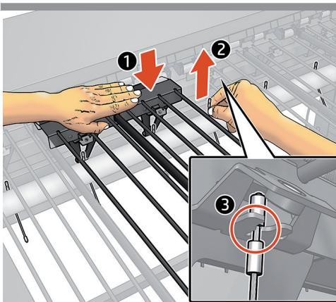
**EN** Push the tray segments down and hook the 6 cables from the tube onto the tray.
