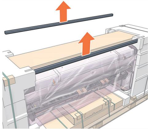
**EN** Remove the adhesive tapes (2 per stand bar), then remove the 2 stand bars.
