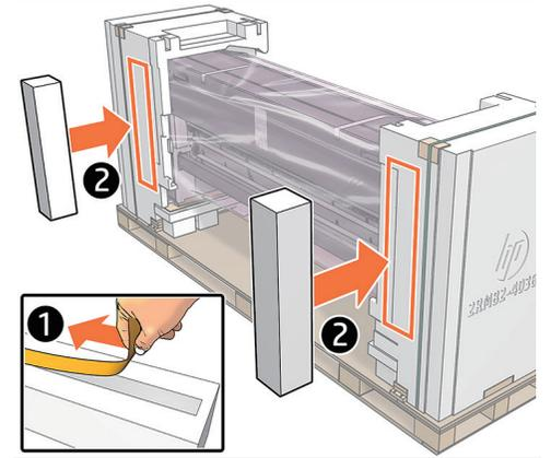
Remove the adhesive tape liners and fix them onto the back of the printer with the 2 adhesive tapes.
