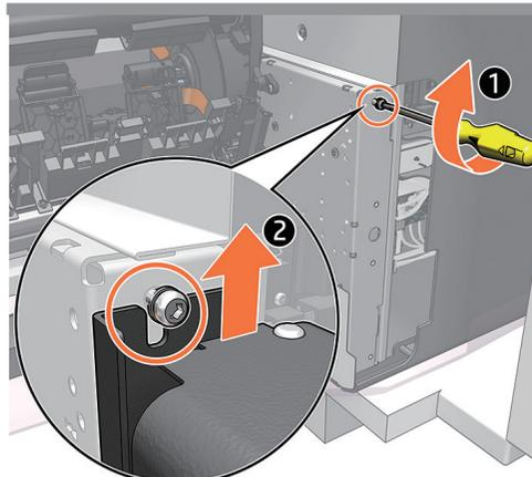
Install the upper screw, but do not fully tighten it, then install the right leg.
