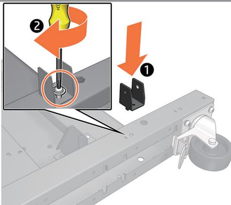
EN Install the sway bar holder at the bottom of left leg and fix it with 1 screw.
