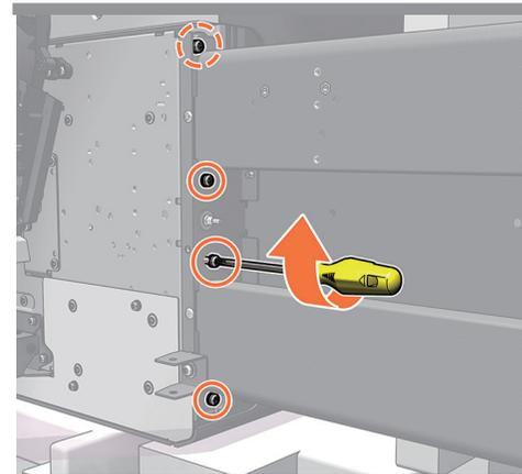
Install the other 3 screws loosely, then fully tighten all 4 screws.
