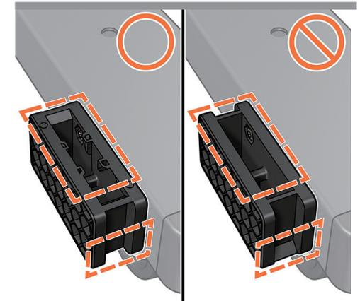
EN Check that the basket holders are correctly assembled.
