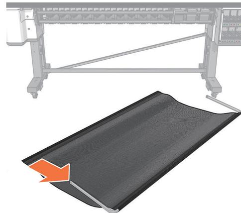
Insert the metallic bar into the fabric on the side without straps.
