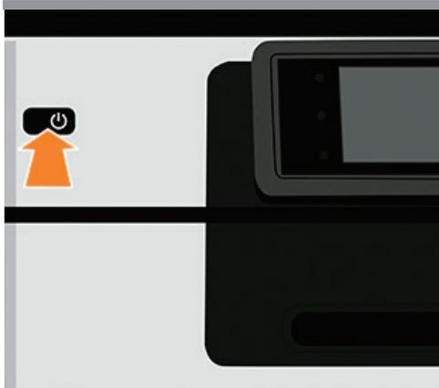
**EN** Switch on the printer next to the front panel.
