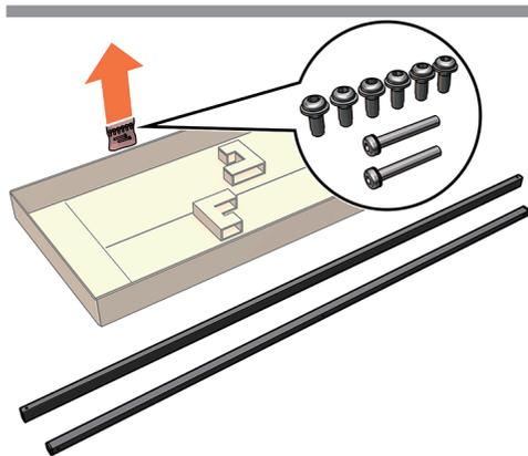
Remove the stand bars and screws from the box.
