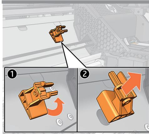
Turn the locker 90° to unplug it from the scan axis beam.
