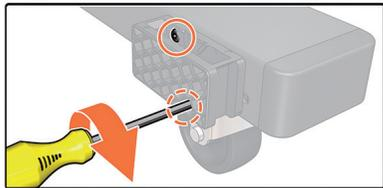
EN Fix the basket holders into place with 2 screws each.
