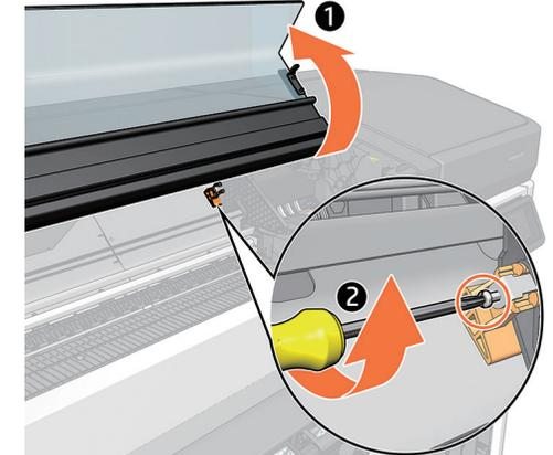
Remove the adhesive tapes, open the window and unscrew (T15) the carriage locker at the right-hand side of the print zone.
