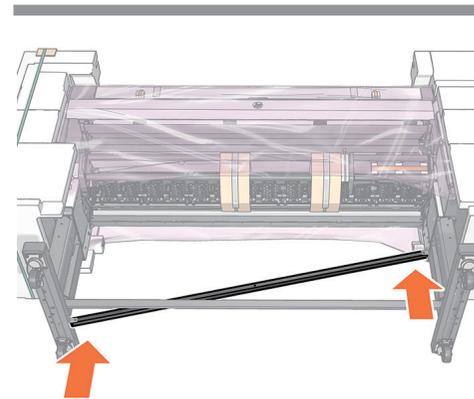
Install the sway bars. **Important:** The head of the center screw must face upwards.
