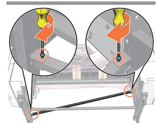
Fix the sway bar into place with the 2 black screws.
