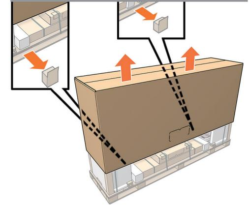
Remove the box, and the 2 wooden blocks from the back of the pallet.
