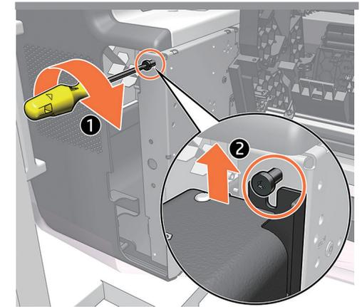
Install the top screw, then install the left leg.
