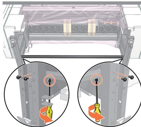
Install the sway bar and fix it to the sway bar holders using 1 screw each side. Make sure all the black screws are fully tightened.
