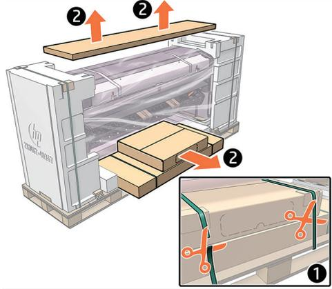
Cut the straps and remove the inbox material, the stand box and the basket box.
