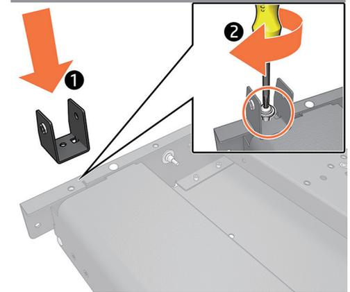
Install the sway bar holder at the top of right leg and fix it with 1 screw.
