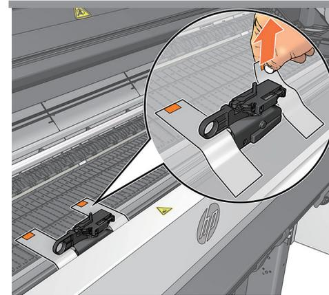
Remove the adhesive tapes from the cutter.
