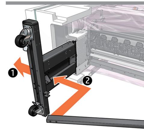
Move the left leg out and place the other end of the crossbar into the left leg slot.
