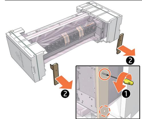
With a T25 screwdriver, remove the 4 screws and the 2 wooden supplements from the bottom.
