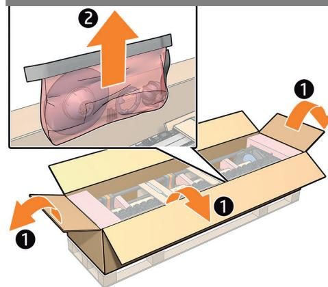
**EN** Remove the bag with the 3-inch accessories and screws.
