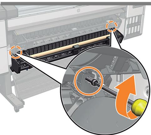
**EN** Fix the multifunction roll with 2xT25 screws.
