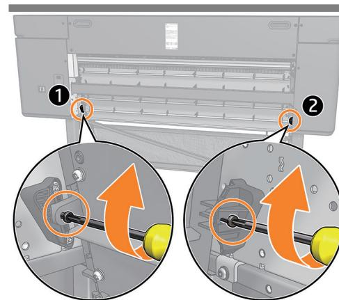
**EN** At the back of the printer, fix in place with a T20 screw on the left (1), and a T20 screw and washer at the right (2).
