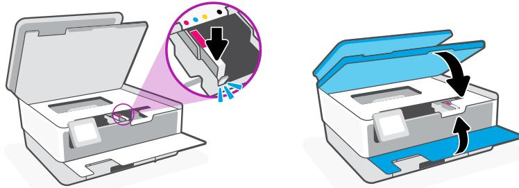
Insert each cartridge securely into the indicated slot. Close both doors.
