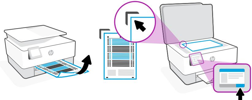
Use the control panel to print and scan the alignment page.
