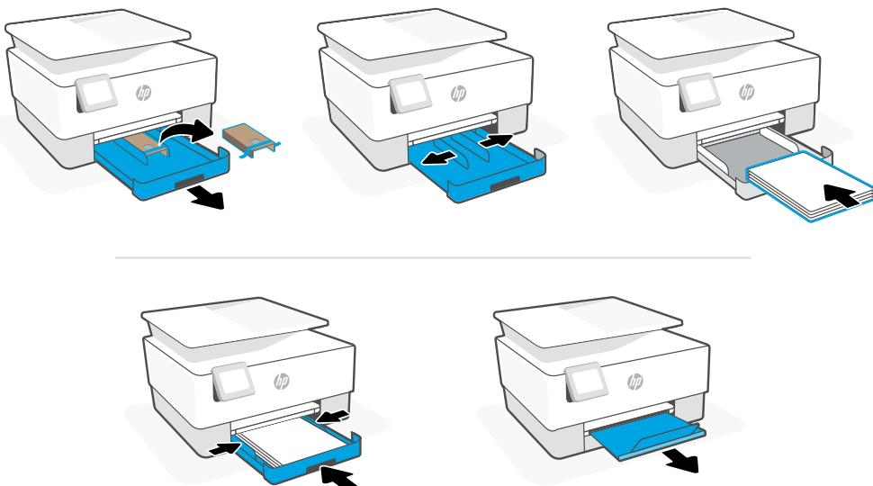
Open the paper tray, remove the cardboard, and slide out the guides. Load Letter or A4 paper and adjust the guides. Close the tray. Pull open the output tray extender.
