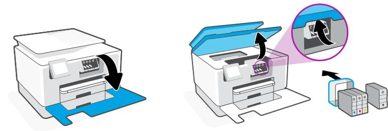
Open the front door and then lift the carriage access door by the scanner lid. Unpack cartridges.
