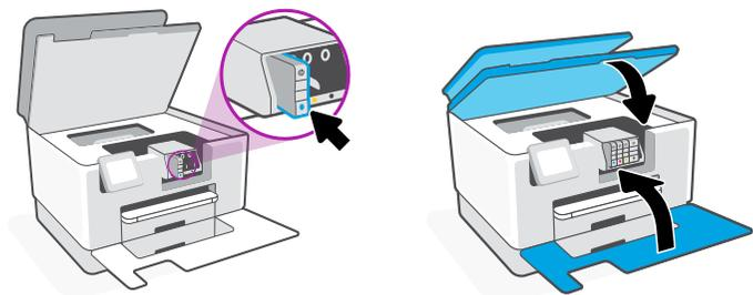
Insert each cartridge securely into the indicated slot. Close both doors.
