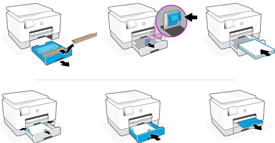
Open the paper tray, remove the cardboard, and slide out the guides. Load Letter or A4 paper and adjust the guides. Close the tray. Pull open the output tray extender.
