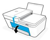
Remove the tape on the outside of the printer. Open the output tray. 打開出紙匣。取下印表機外部的膠帶。
