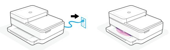
Plug in to automatically power on. Wait until the printer lighting is purple before continuing. Do not connect a USB cable during setup.
