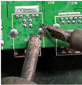
USB upstream connector repairing
