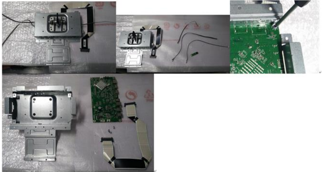
PCBA and chassis separate step
