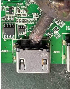
HDMI connector repairing
