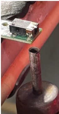
Headphone connector repairing
