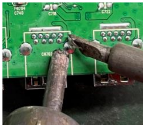
USB connector repairing
