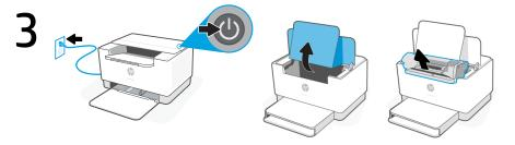
Power off the **original printer** and remove the power cord from the wall outlet, open access door and remove toner cartridge and install toner in your replacement printer along with all other accessories
