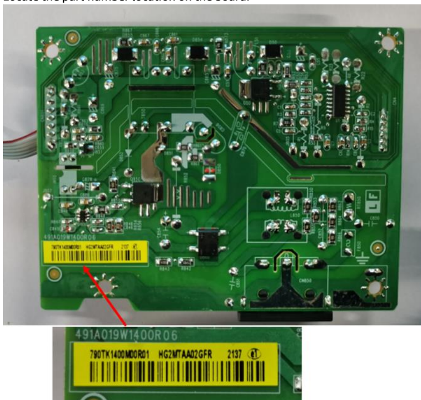
Part number location of power board
