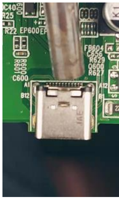
Remove USB-C connector
