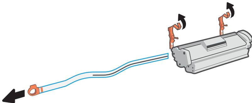
**EN** Remove the orange guides and tape. Pull the tab to remove the protective film completely from the cartridge.
