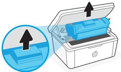
**EN** Remove the cartridge from the printer.
