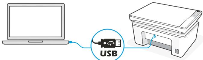
**EN** Connect the printer to a computer using a USB cable.
