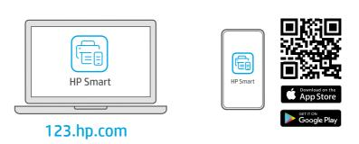
Install the **required** HP Smart software from **123.hp.com** or your app store on a computer or mobile device.
