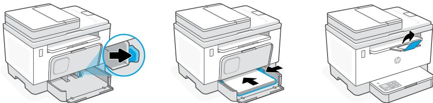
**EN** Adjust guides and load paper. Open the output tray extender.
