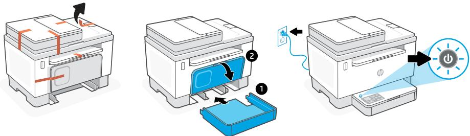
**EN** Remove all tape and slide the tray into place. Plug in and power on the printer.
