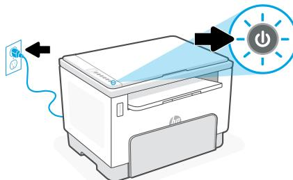
**EN** Remove all packaging and tape. Plug in and power on the printer.
