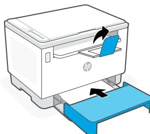
**EN** Adjust guides, load paper and slide the tray cover into place. Open the output tray extender.
