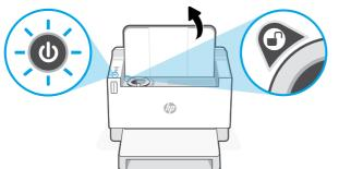
Toner can be added only when the port indicator shows an **unlock** icon ( ). For more information, see the User Guide at hp.com/support
