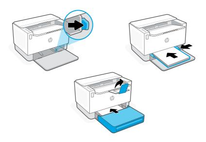
Adjust guides, load paper and slide the tray cover into place. Open the output tray extender.
