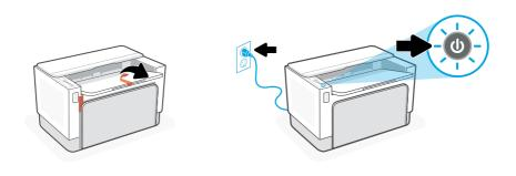
Remove all packaging and tape. Plug in and power on the printer.
