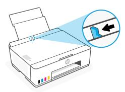
2. Load new, unused Letter or A4 paper, and adjust the paper guide. Open the output tray extender.
