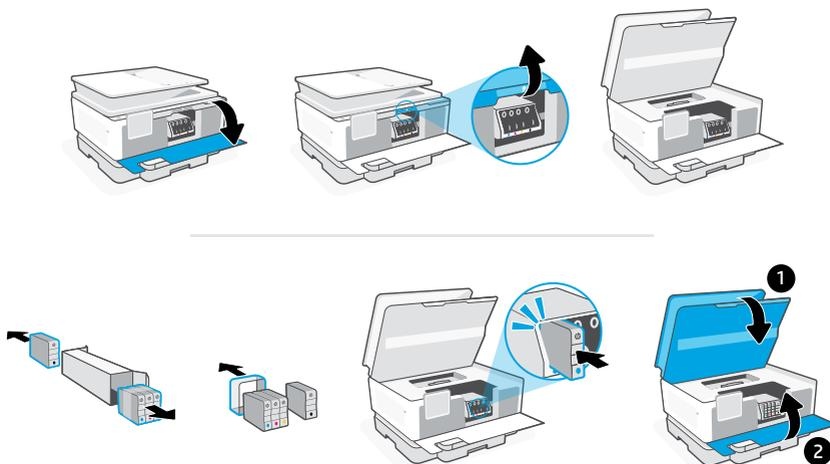
**EN** Open the front door and then lift the cartridge access door by the scanner lid. Unpack cartridges. Insert each cartridge securely into the indicated slot. Close both doors.
