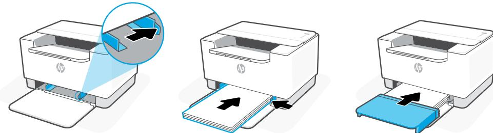
**EN** Slide out the guides. Load Letter or A4 paper and adjust the guides. Slide the tray cover into place.
